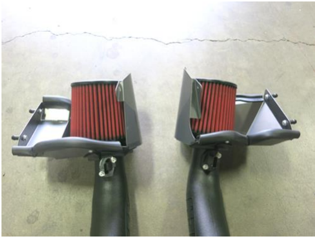
f. Pull the tubes so the MAF mounts are on the outside of the heatshields and install the MAF sensors using the factory hardware.
