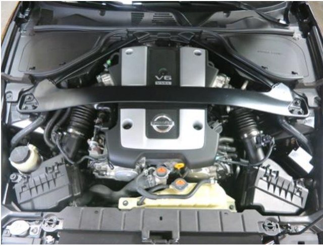
STOCK INTAKE INSTALLED
