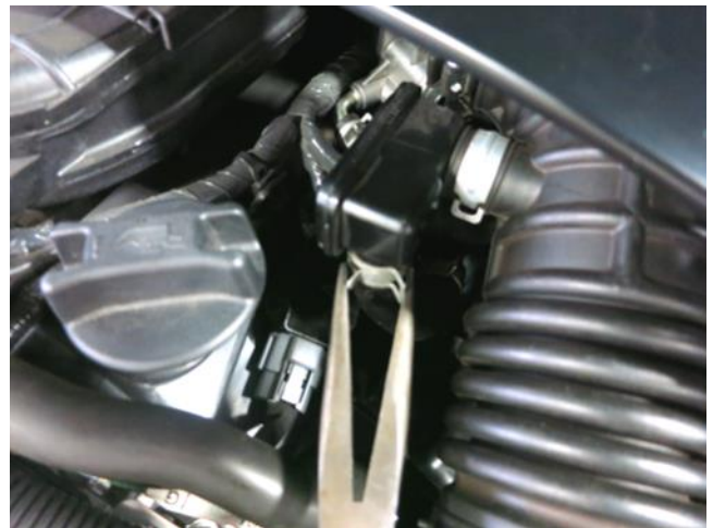
d. Disconnect the PCV hose on the driver side by releasing pressure on the spring clamp.
