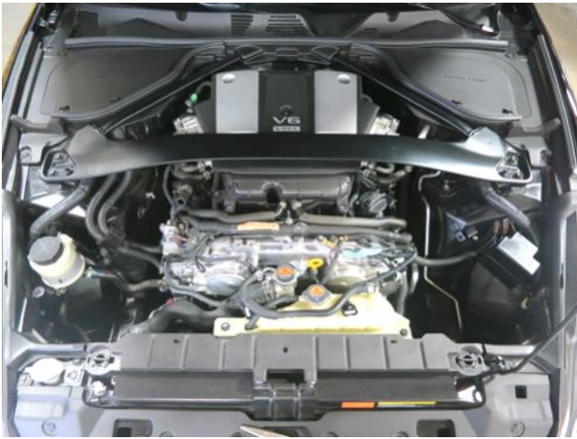
g. Lift each air box up and out of the vehicle, releasing them from their grommets. Then, remove the air hoses.
