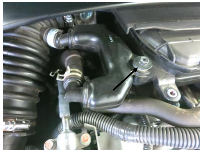
b. Remove the bolt securing the PCV hose fitting on the passenger side.
