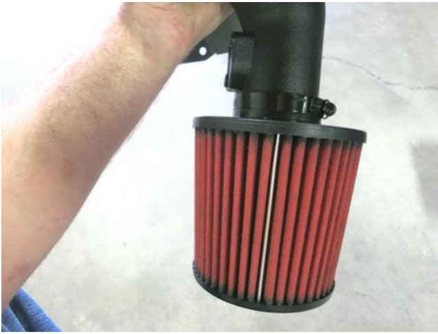
e. With the tube inserted through the heatshield, install the AEM Dryflow filter onto the tube using the MAF mount and filter media clip as a reference as shown.
