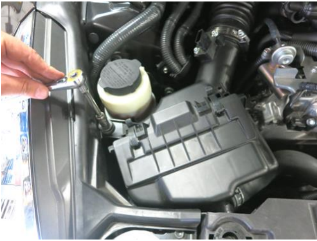
e. Remove the bolts securing the factory air box on each side of the vehicle.
