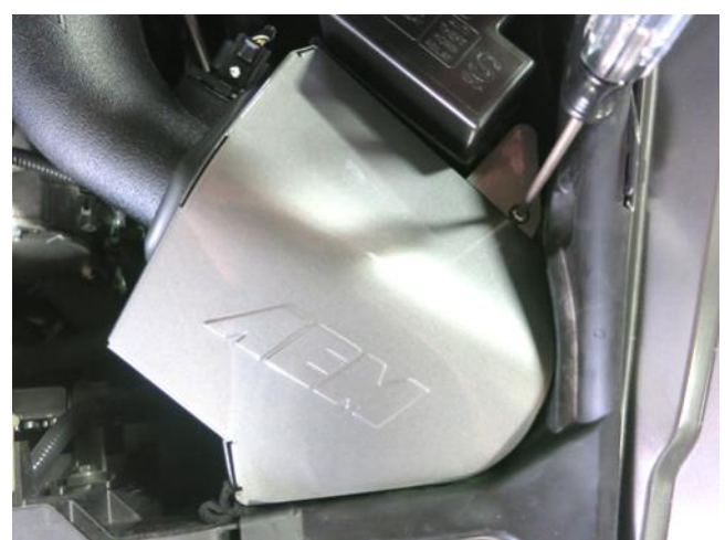
n. Pull the driver side heatshield into position and secure with the provided hardware. Ensure the fuse box latch is below the heatshield lip.
