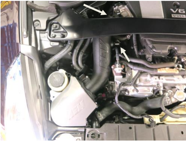
k. Push the passenger side heatshield down into the grommets as shown. Then, connect the PCV hose and secure it with the spring clamp. Then, insert the tube into the coupler.
