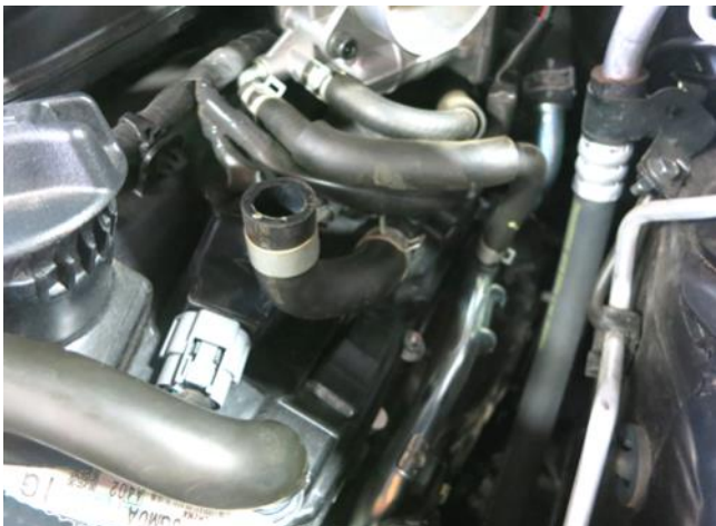
h. Install the PCV hose removed in step 2i, reversing its orientation as shown.
