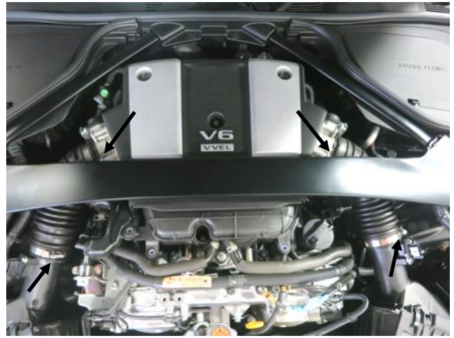
f. Loosen the four hose clamps on the factory air hoses.
