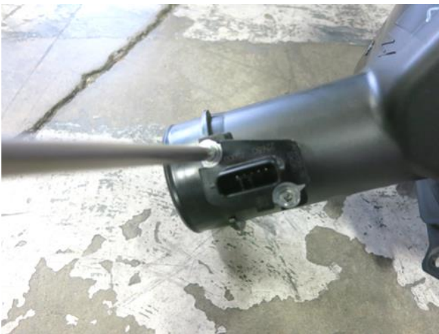
o. Remove both MAF sensors from their factory air boxes. Note: Do not discard any of your stock equipment.
