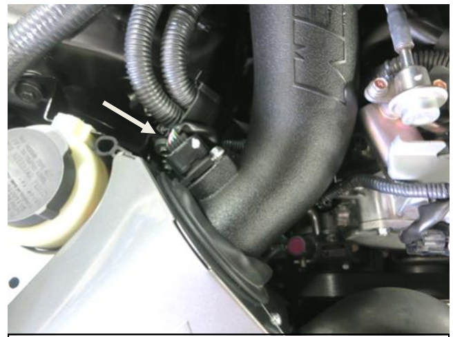
n. Route the MAF harness under each tube and connect the harness to the sensor on each side of the vehicle.
