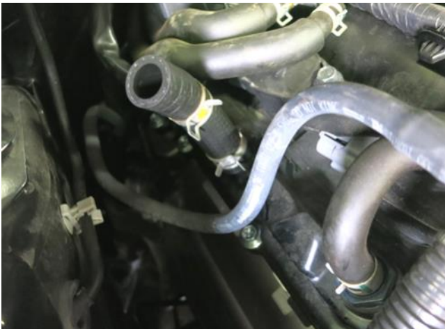
g. Install the provided hose using the factory spring clamps on the passenger side valve cover.
