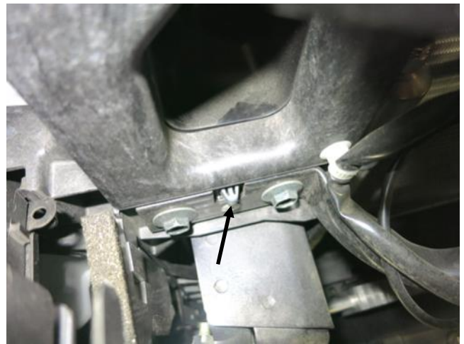
n. Use needle nose pliers to squeeze the retaining clip to release the air ducting on both sides of the vehicle. Remove the air ducting.
