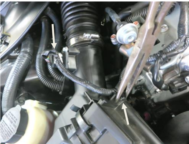
c. Release the Mass Air Flow (MAF) sensor harness and disconnect the connector on both sides of the vehicle.
