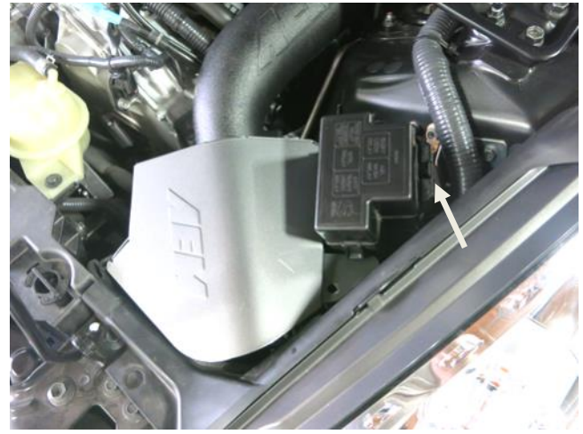
l. The fuse box on the driver side can be released to aid in installation by depressing the clip. Seat the heatshield into the grommets and then replace the fuse box.
