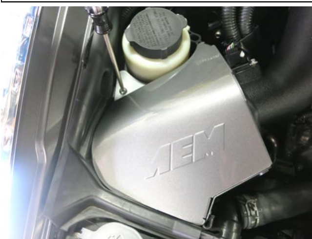
n. Pull the passenger side heatshield into position and secure with the provided hardware. The heatshield should clear the power steering reservoir and the power steering hose should route through the cutout.
