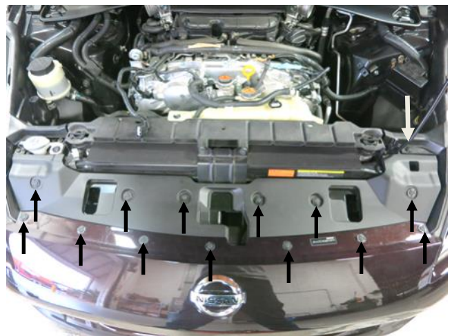
j. Remove the 14 plastic push-rivets and then remove the plastic radiator shroud. Note: The push-rivet denoted by a white arrow is a unique size.
