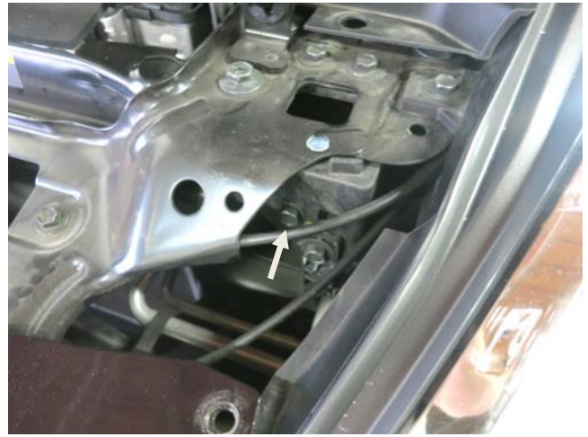
l. Remove the bolt securing the driver side air ducting.
