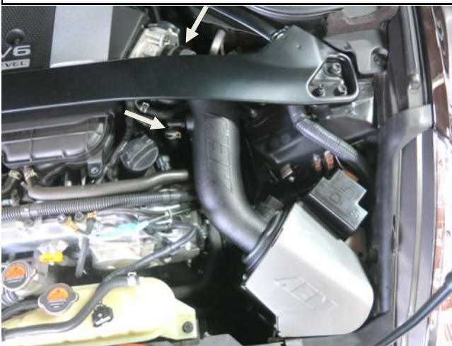
m. Connect the PCV hose and insert the tube into the coupler. Secure the PCV hose with the spring clamp at this time.
