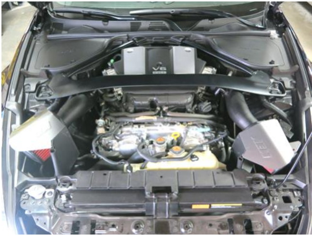
j. Install the tube and heatshield assemblies as shown, maneuvering the tubes under the strut tower brace first. Do not insert the tubes into the couplers until the heatshields are in position and seated into the grommets.
