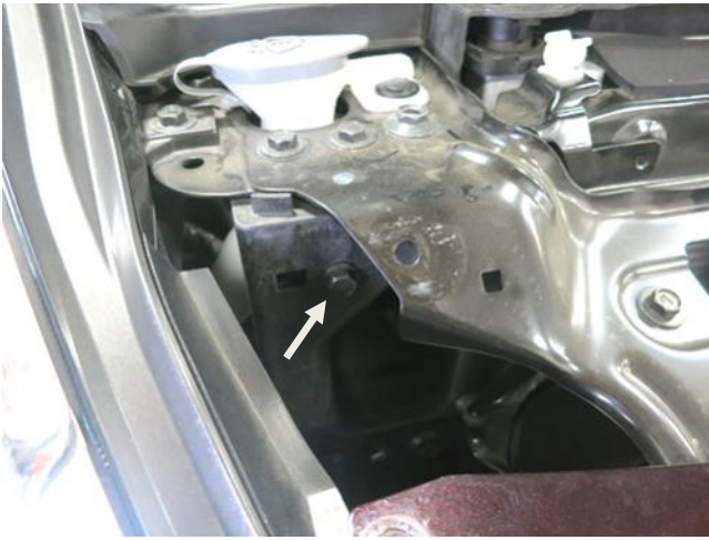
k. Remove the bolt securing the passenger side air ducting.
