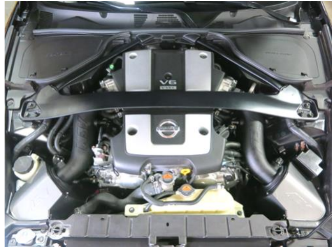
AEM INTAKE INSTALLED
