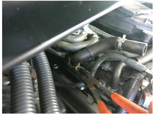
h. Remove the passenger side PCV hose. Remove the hose clamps; these will be used later.
