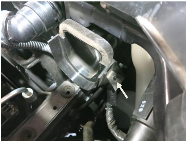
m. Release the wiring harness from the passenger side air ducting.
