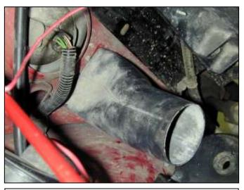
f. Remove the inlet air duct from below the headlight housing.
