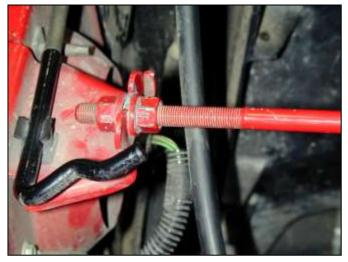
h. Loosen the nuts on the radiator support brace and lift brace off of mount. Rotate the brace out of the engine compartment.
