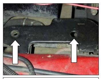
g. Remove the two rubber grommets from the air filter housing mount.
