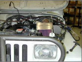
AEM® intake system installed
