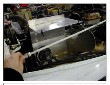
f. Install the heat shield by moving the radiator support bracket out of the way and aligning the holes in the bottom of the heat shield and stock air box bracket.
