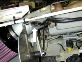
k. Attach the factor charcoal box breather line to the lower intake pipe by sliding it over the nipple.
