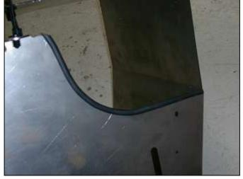
e. Install rubber edge trim onto heat shield and trim to fit.
