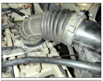
b. Loosen the plastic hose clamps on the rubber intake tube attached to the throttle body. Do this by pulling the two plastic tabs on the hose clamp apart. Disconnect the intake tube from the throttle body.
