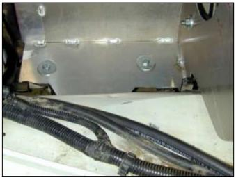
g. Install the two bolts, two nuts, and four washers to secure the bottom of the heat shield. Tighten until nut is snug but do not over tighten.
