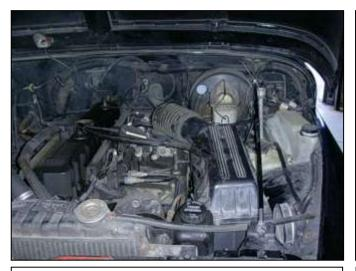
Factory air box system installed
