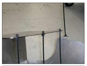
d. Install the plastic zip-tie mounts by pressing them into the holes on the heat shield tab and cover.
