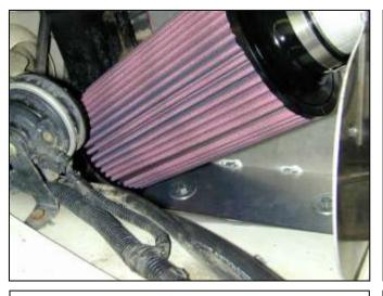
j. Install the AEM<sup>®</sup> air filter into the space behind the headlight. Push the filter over the inlet pipe until the stop in the filter is reached, and then install one hose clamp to secure the filter onto the inlet pipe.
