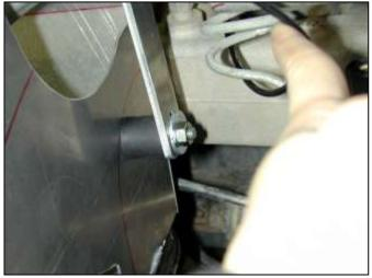
i. Align the intake pipe bracket with the rubber mount on the heat shield. Install the washer and nylok nut onto the rubber mount to capture the bracket.
