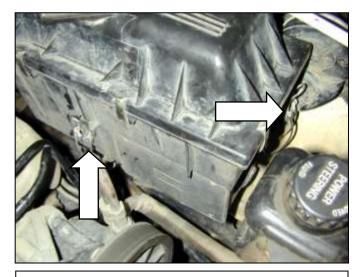
e. Un-clip the three hooks holding the air filter housing to the chassis. Lift the air filter housing and intake tube from the vehicle.
