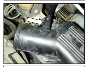
c. Disconnect the charcoal box breather hose from the air filter housing.
