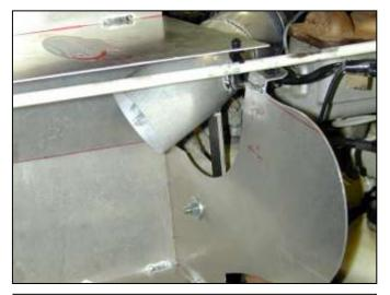
h. Ensure the intake pipe is free from debris. Install the AEM<sup>®</sup> intake pipe into the elbow on the throttle body. This is to be installed with the small bend towards the elbow.
