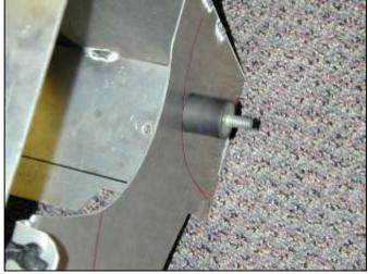
c. Prepare the heat shield for installation by first installing the rubber mount into the slot as shown.
