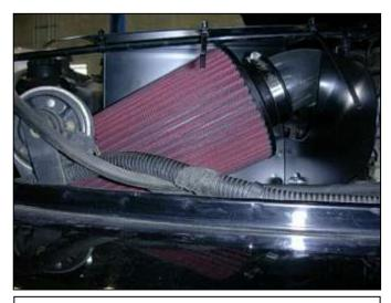
n. Ensure that the air filter is not touching any part of the vehicle. Position the AEM<sup>®</sup> intake system for best fitment. Be sure that the pipe or any other component is not in contact with any part of the vehicle. Tighten the hose clamps at the throttle body. Tighten the nut on the mounting bracket. Readjust pipe if necessary. Install rubber edge trim to the top of the heat shield
