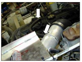
I. Install the supplied 1/2" breather hose between the intake pipe nipple and the valve cover elbow using two 1-1/16" hose clamps.
