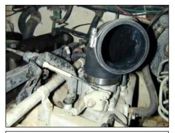
b. Install the rubber elbow with the smaller, 2.5" side on the throttle body. Attach elbow using the supplied #44 Hose clamp.
