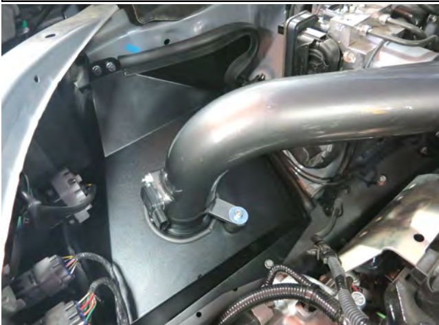
g. Carefully lower the assembly into the engine bay. It will take some maneuvering to seat the heatshield assembly into place. Fasten using the provided bolt and the nuts removed in step 2g.
