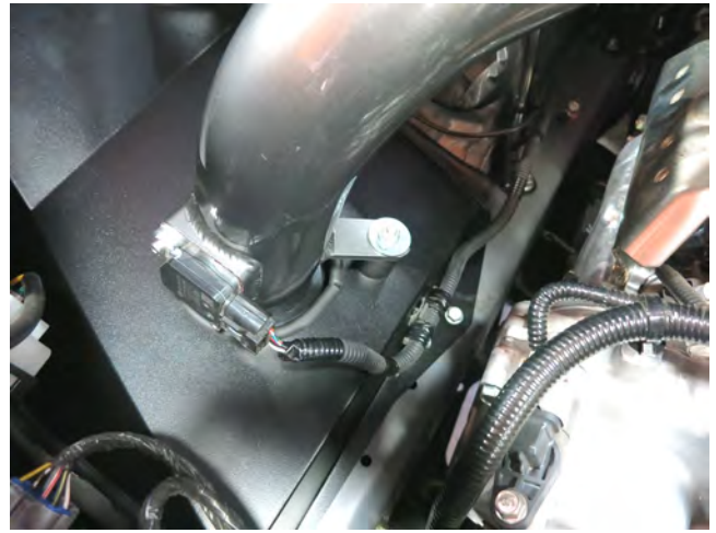
j. Connect the MAF sensor harness to the MAF sensor and secure the harness on the heatshield. Tighten the nut on the bracket to secure the tube.
