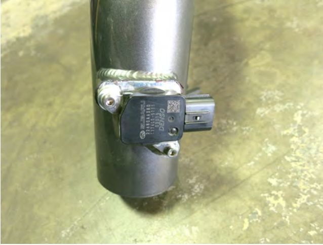
a. Install the MAF sensor into the AEM intake tube using the provided hardware.
