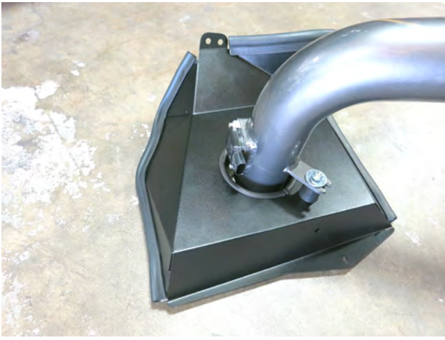
e. Install the intake tube as shown, sliding the bracket below the washer on the rubber mount. Do not fully tighten the nut to allow some movement during installation.
