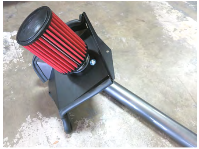
f. Install the AEM DryFlow filter using the provided hose clamp onto the intake tube.
