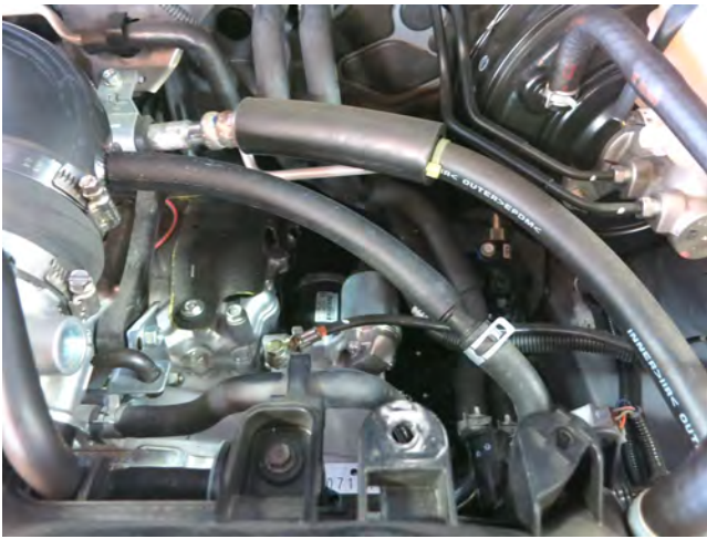
i. Connect the factory PCV hose to the supplied hose and secure using the factory spring clamp.
