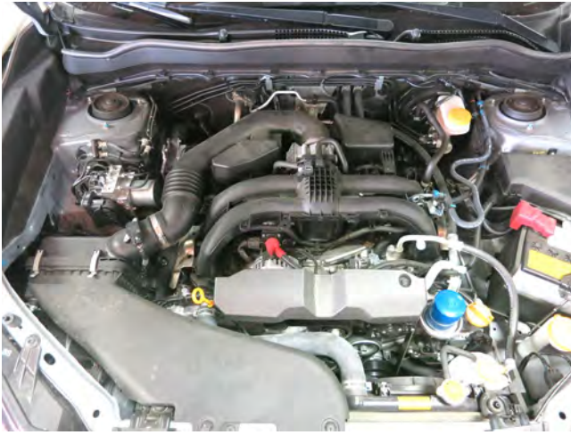
STOCK INTAKE INSTALLED
