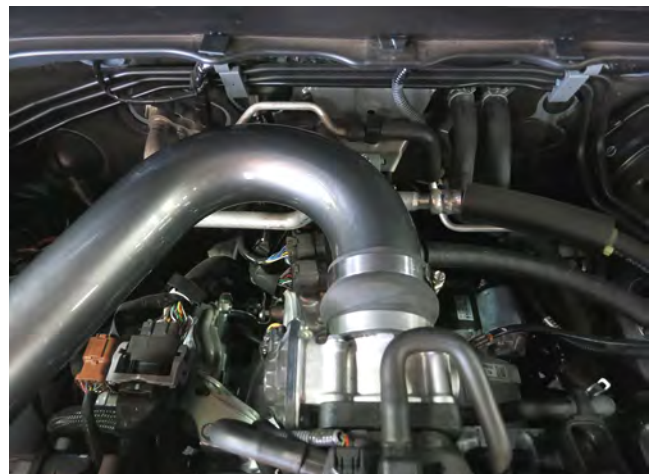
h. Insert the intake tube into the coupler. Position the tube for best fit and tighten the hose clamp.
