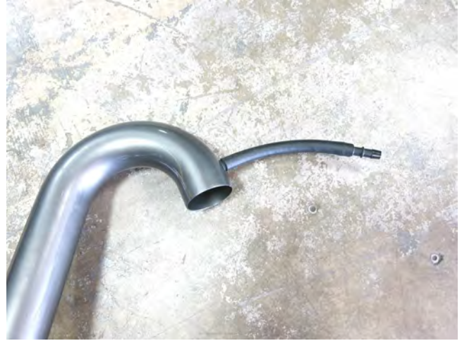
b. Attach the provided hose and hose fitting to the intake tube nipple.
