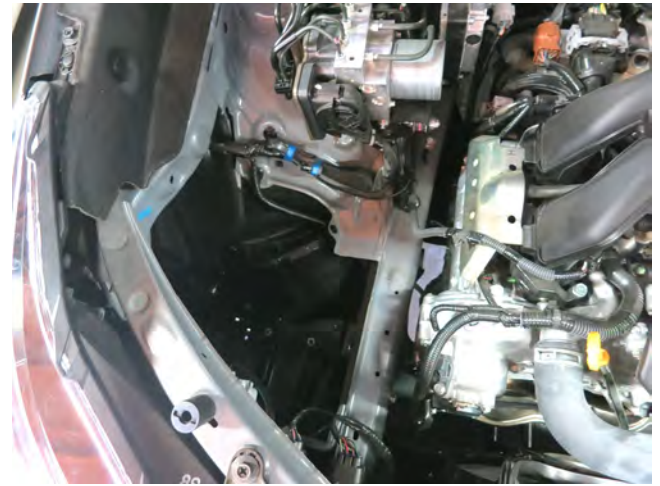
h. Lift the air box up and out of the engine bay. Tuck the MAF sensor harness towards the engine so it is out of the way.
