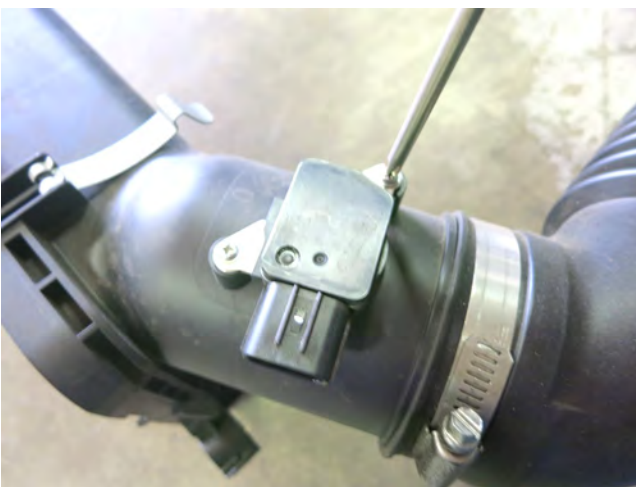
i. Remove the MAF sensor from the air box lid assembly. Replace the screws into the air box lid for safe keeping. Do not discard any of your stock equipment.
