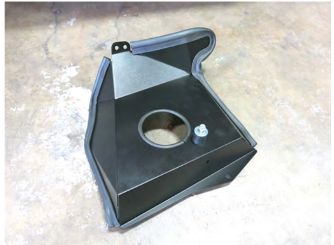
d. Install the edge trim onto the heat shield as shown. Install the rubber mount using the provided hardware. Leave the top nut and washer loose to aid in installation of the intake tube.
