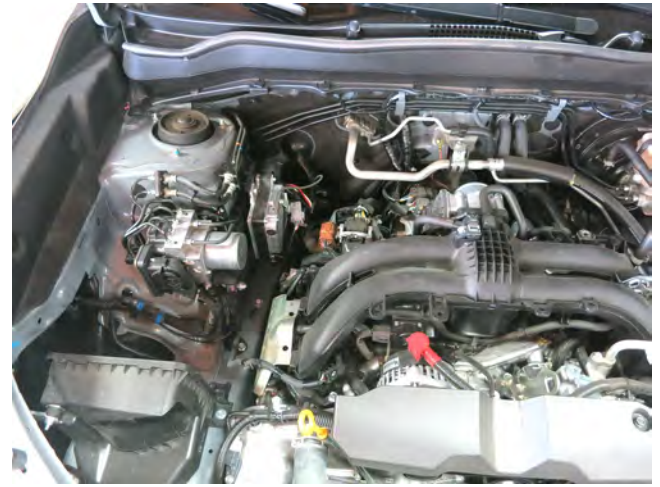
f. Unlatch the air box lid and remove the air box lid and intake resonator assembly out of the engine bay.
