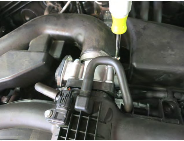
e. Loosen the hose clamp securing the factory intake to the throttle body.
