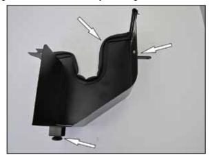
7. Install the factory mounting grommet, mounting bracket (064356) and edge trim onto the heat
