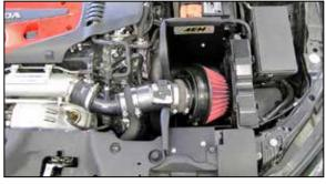
13. Install the intake tube assembly onto the turbo inlet, adjust the assembly for best fit and then secure with the provided hose clamp.
