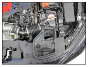
2. Disconnect the mass air sensor electrical connection and unhook the wiring harness from the air filter housing.
