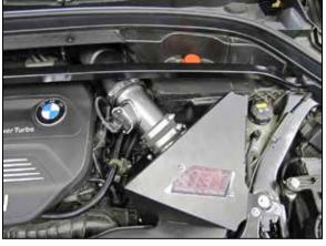
11. Install the provided coupler onto the intake tube but do not secure. Install the intake tube assembly into the factory intake hose and align with the filter adapter, slide the coupler onto the adapter and adjust the assembly for best fit. Secure the intake tube assembly with the provided hose clamps. Beconnect the mass air sensor electrical
