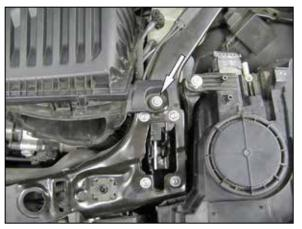
4. Remove the bolt that secures air filter housing to the core support.
