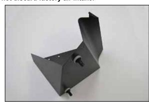
6. Install the provided mounting studs to the heat shield as shown.
