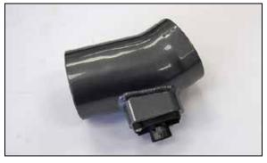
10. Remove the mas air sensor from the factory housing and install it into the AEM<sup>®</sup> intake tube using the hardware provided.
