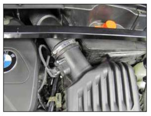
2. Disconnect the mass air sensor electrical connection and disconnect the wiring harness from the air filter housing.
