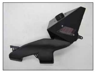
8. Install the AEM<sup>®</sup> badge into the upper air filter housing and then assemble the two filter housing halves and fresh air scoop and secure with the provided hardware.
