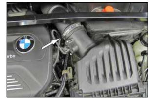
5. Loosen the hose clamp that secures the intake hose to the air filter housing then remove the air filter housing from the vehicle. **NOTE: AEM recommends that customers do not discard factory air intake.**
