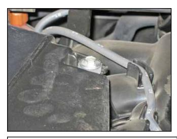
f. Remove the bolt securing the stock intake system to the intake manifold.
