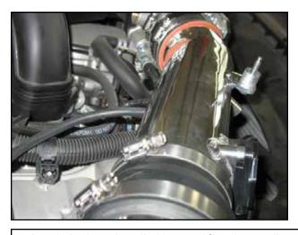
q. Attach the hose installed in step 3f. to the small nipple located on the back of the intake pipe.
