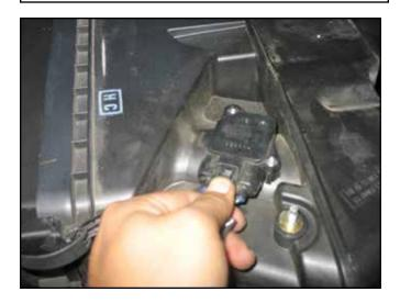
c. Disconnect the Mass Air Flow (MAF) sensor.
