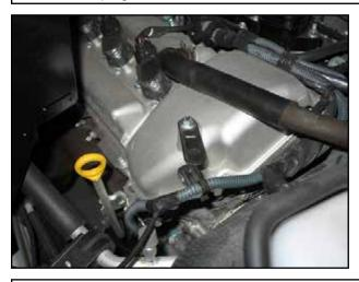
d. Secure the supplied stainless steel bracket to the valve cover using supplied bolt and washer.
