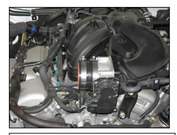
I. Install the coupler loosely at the throttle body using the supplied #48 hose clamps.
