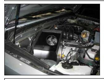
h. Prepare the heat shield with edge trim and rubber gasket then place in the engine bay as shown.
