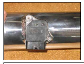
c. Install mass air flow sensor in pipe using supplied bolts.
