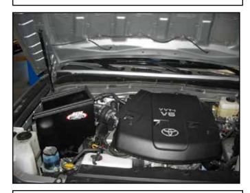
AEM® intake system installed
