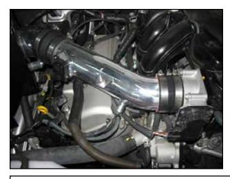
p. Use the supplied 8mm washer and serrated nut to secure the lower pipe to the rubber mount.
