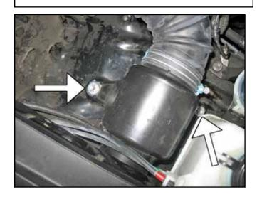
h. Remove the two bolts that secure the intake tube to the fender well.
