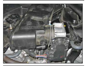
i. Loosen the hose clamp securing the stock air box to the throttle body.
