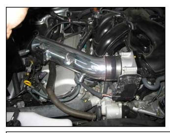
m. Insert the upper pipe into the coupler at the throttle body.
