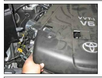
n. Line up the bolt that is attached to your upper intake pipe with the hole on the engine cover, then remove the engine cover again.
