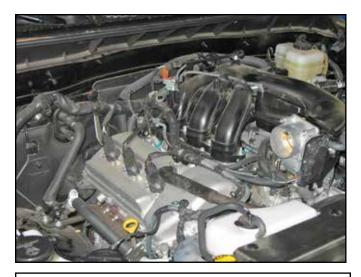
k. Factory air box completely removed from vehicle.
