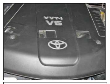
b. Remove two nuts securing the engine cover to the intake system and engine.
