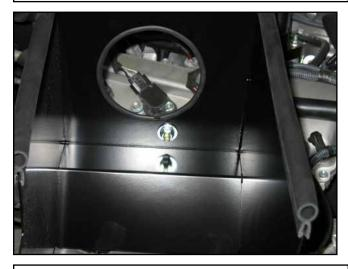
k. Install the rubber mount in the heat shield with the supplied 8mm washer and serrated nut.
