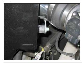
o. Install the screened hose adapter to the end of the upper pipe and guide the lower pipe through the heat shield, while lining up the bracket with the rubber mount as well.
