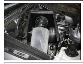
s. Install filter on the end of the lower pipe.
