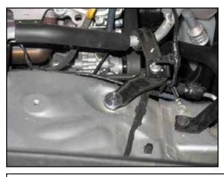
g. Place the supplied spacer on top of the A/C line bracket. Lining it up with the hole beneath it.
