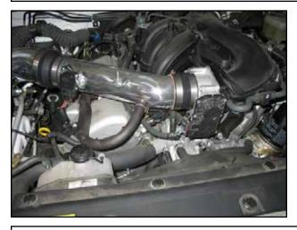
r. Reattach the PCV hose to the nipple on the upper pipe using the stock hose clamp. Also plug the MAF sensor back in.
