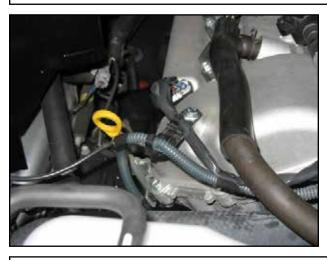
e. Attach the zip ties that we removed from the stock intake system to the previously installed bracket.
