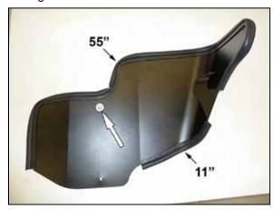
11. Install the edge trim onto the heat shield as shown. Install the rubber mounted stud into the top hole of the heat shield.
