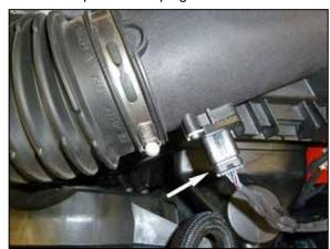
8. Disconnect the mass air sensor electrical connection.
