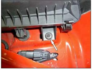
9. Remove the bolt that secures the air filter housing to the inner fender. Lift the air filter housing up to dislodge it from the mounting grommet and then remove the complete system from the vehicle. NOTE: AEM recommends that customers do not discard factory air intake.
