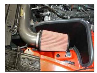
17. Install the AEM® air filter onto the intake tube and secure with the provided hose clamp.
