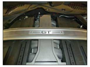
2. Remove the four nuts that secure the strut brace and then remove the strut brace from the vehicle.
