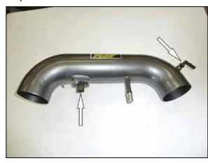
14. Remove the mass air sensor from the factory air filter housing and install it into the AEM® intake tube using the provided hardware. Install the 90° NPT fitting as shown.
