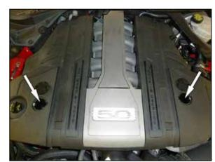
3. Pop up the two-round bolt covers and then remove the two nuts that secure the decorative engine cover and remove the cover from the engine.
