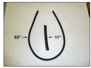
10. Cut the provided edge trim into two sections, one section will be 11" long and one section will be 55" long.
