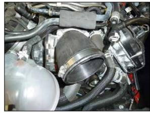
13. Install the provided coupler (5-1100) onto the throttle body and secure with the provided hose clamp.
