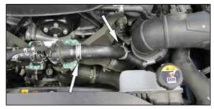
4. Release the spring clamps that secure the driver side BOV hose to the BOV and intake tube, then remove the driver side BOV hose. **NOTE: This hose will be reused.**  5. Loosen the hose clamps that secure the intake tube to the air filter housing and turbo inlet and then remove the intake tube from the vehicle.
