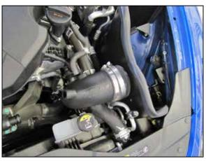
12. Install the driver's side heat shield assembly into the vehicle and secure with the provided hardware. Then install the intake tube assembly onto the turbo inlet.
