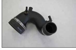
10. Install the provided couplers (5-222N & 08761) onto the Drivers side intake tube (9-0459) and then
