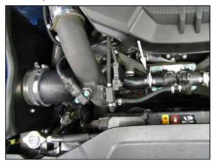
19. Install the driver's side BOV hose and secure with the factory hose clamps. NOTE: Some trimming of the BOV hose may be necessary to avoid kinks in the hose.
