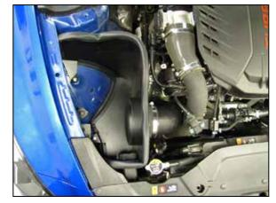
18. Install the provided filter adapter into the heat shield so that it goes through the heat shield and into the coupler on the intake tube. Secure the adapter to the heat shield using the provided hardware and then adjust the intake tube and couplers for best fit and secure with the provided hose clamps.
