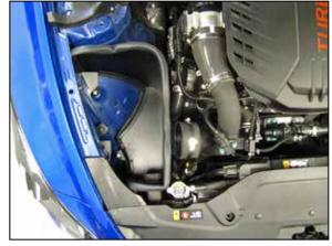
17. Install the passenger side heat shield and secure with the provided hardware.
