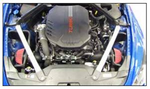
21. Reinstall both strut tower braces and secure with the factory hardware.
