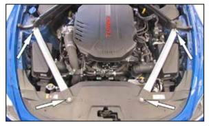
2. Remove the four bolts shown that secure the two strut tower braces to the vehicle and then remove the braces from the vehicle. **NOTE: These braces and bolts will be**
