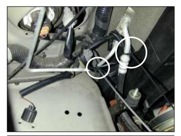
I. Use the included zip-ties to tuck the extra wires that are behind the headlight out of the way. This will keep the wires from interfering with the air filter.
