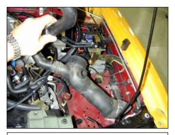
j. Unsnap the ducting assembly from the inner fender and remove it from the engine bay.
