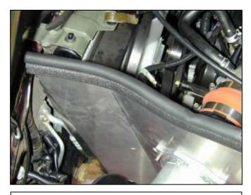
s. Push the molding onto the upper edge of the heat shield as shown in the picture.
