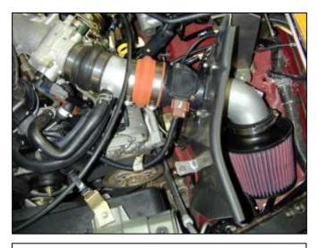
t. Check final fitment of the intake system and heat shield. Make sure no part of the intake system makes contact with the vehicle. After adjusting the position of the system, tighten down the mounting nuts on the heat shield and all of the hose clamps.
