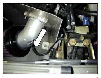
p. Install the included 3/16" hose between the connector on the pipe and the vacuum solenoid.
