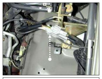
m. Bend the wire plug holders as shown in the picture, this will allow additional clearance for the heat shield.
