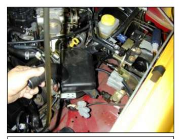
f. Remove any wiring harnesses attached to the resonator chamber and remove from the engine bay. PLUG IN THE WIRES that were unplugged in the previous step after the chamber was removed.
