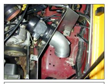
f. Place the assembly from step 3(d) into the engine bay as shown in the picture. Line up the tabs of the heat shield with the rubber mount studs.
