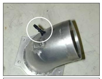
c. Insert the rubber grommet and vacuum hose connector into the small hole on the MAF sensor adaptor pipe. On vehicles not equipped with vacuum solenoid use vacuum cap to seal off vacuum hose connector first then install into grommet.
