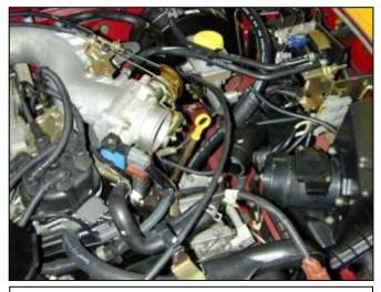
b. Remove the factory intake hose from the engine bay.
