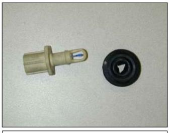
h. Remove the rubber grommet from the IAT sensor.
