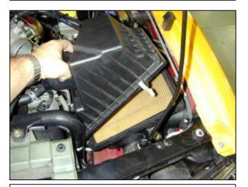
c. Undo the four snaps located around the perimeter of the air filter housing box. Unplug the small vacuum hose on the vacuum solenoid. Remove the top lid and the air filter.
