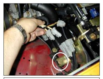
e. Remove the fastener circled in the picture. Unplug the three wiring connectors shown in the picture. This will allow easier access to the intake resonator chamber.
