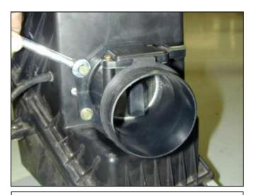
k. Remove the MAF sensor from the air box by removing the four mounting bolts.
