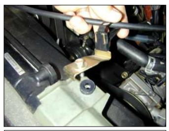
b. Place the supplied round spacer underneath the throttle cable bracket as shown. Secure the bracket in place by reusing one of the fasteners from step 2(i). Skip this step for normally aspirated vehicles.
