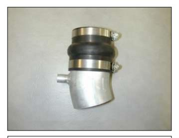
k. Insert the 2.75"-3.0" hump hose reducer on to the throttle body end of the pipe with the 3.0" end around the pipe. Use a #48 hose clamp for the 3" end and a #44 hose clamp around the 2.75" end.
