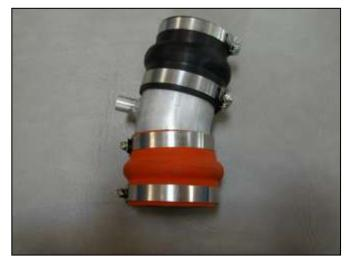
I. Place the 3" hump hose and #48 hose clamps around the other end of the pipe as shown.
