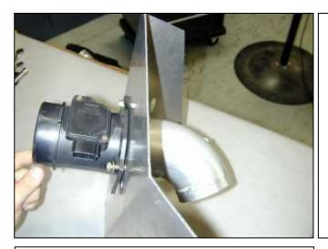
d. Create the assembly shown in the picture by following the diagram below. Make sure the AEM<sup>®</sup> pipe is oriented so that it angles downward. **Be** sure not to overtighten the MAF sensor bolts, this will damage the threads in the aluminum adaptor and possibly the MAF sensor.
