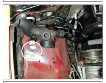
h. Remove the two bolts and the bracket circled in the picture.
