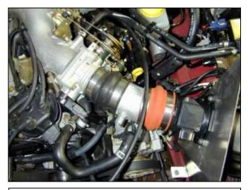
n. Place the assembly from the previous step into the vehicle with the 2.75" hose around the throttle body and the 3" end around the MAF sensor. Make sure the nipples are facing toward the front of the vehicle.
