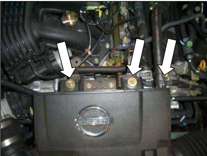
c. Loosen and remove the mounting bolts for the combination resonator chamber and inlet tube. Remove the crank case breather tube from the resonator housing.
