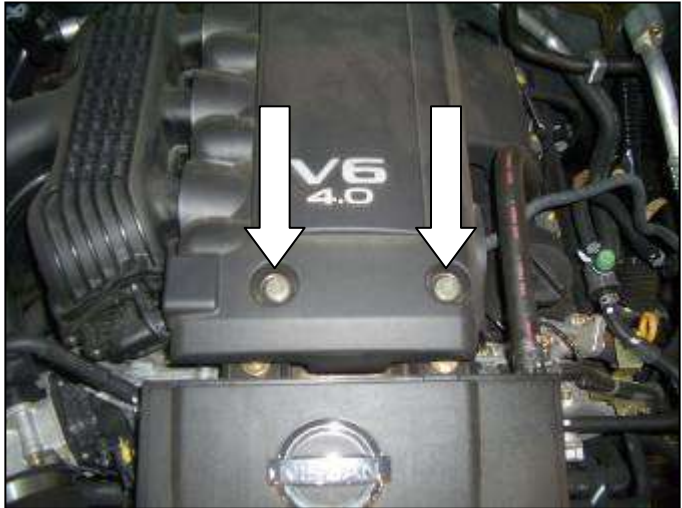
b. Loosen and remove the two bolts to the engine cover. The cover is held in place with two rubber isolators, one on each side. Remove the engine cover by pulling straight up.
