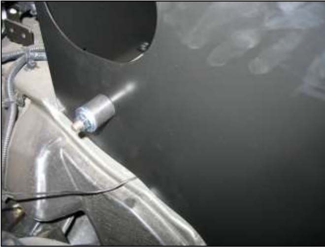
f. Insert and secure the rubber mount through the heat shield with the provided hardware.
