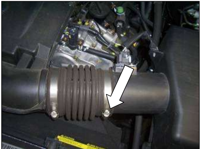
d. Loosen the hose clamp securing the inlet tube to the air box. Remove the combination resonator chamber and inlet tube.
