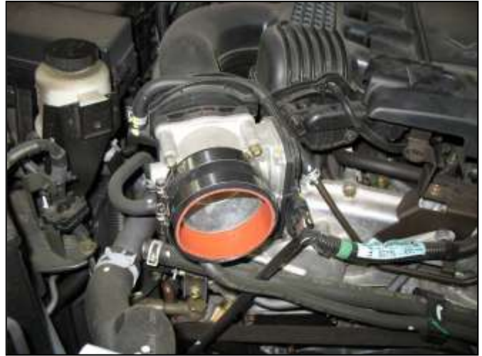
g. Attach and secure the coupler to the throttle body with the provided hose clamps.
