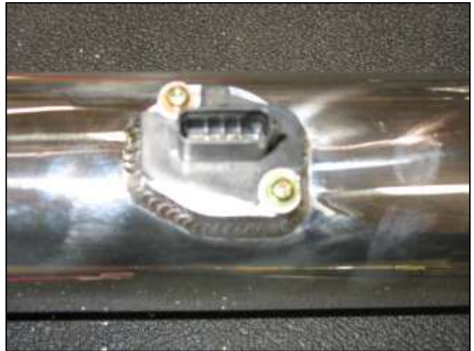
i. Install the MAF sensor (removed in step 2g) into the intake pipe.
