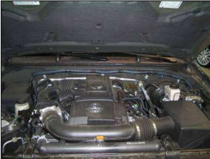
a. Stock air box system installed. Loosen hose clamps securing inlet tube to the throttle body.
