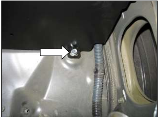
e. Use the stock threaded hole location to secure the heat shield as shown.
