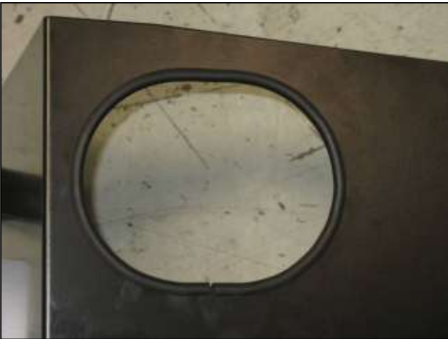
h. Attach rubber edge trim around the intake pipe opening of the heat shield.
