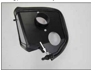
12. Install the mounting post from the previous step onto the  $AEM^{\otimes}$  heat shield as shown.
