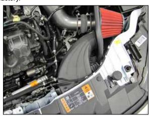
24. Install the AEM® fresh air duct into the heat shield and core support as shown and secure with the two provided retaining clips.
