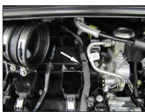
16. Unhook the wiring harness clip from the mounting stud, route the harness next to the coil and fuel line and secure the harness to the fuel line with the provided tie wrap.
