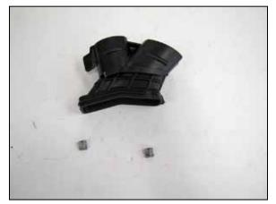
22. Remove the two clips from the factory inlet air
