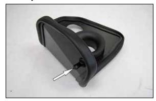
10. Install the heat shield mounting stud onto the heat shield and secure with the provided hardware.
