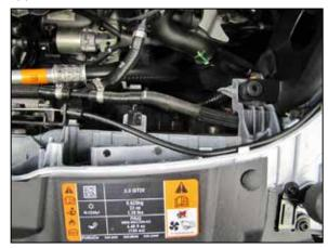
21. Using the Fresh air duct as a guide, mark the two hole locations onto the fresh air duct in the core support. Next remove the AEM® fresh air duct and drill two 1/4"id holes into the factory fresh air duct at the marked locations.
