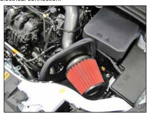
19. Install the AEM® air filter onto the filter adapter and secure with the provided hose clamp.
