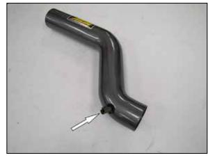
15. Install the grommet provided and the factory inlet air temperature sensor into the AEM® intake tube as shown.
