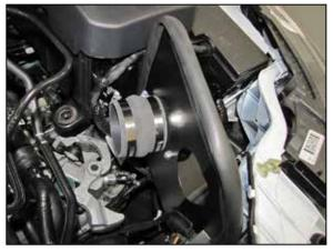
14. Install the provided coupler hose (087121) onto the filter adapter and secure with the provided hose clamp.
