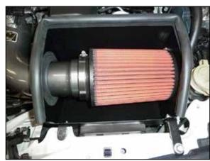
22. Install the air filter onto the AEM® intake tube and secure with the provided hose clamp.
