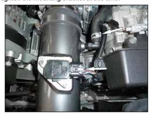
20. Connect the crank case vent to the fitting installed into the AEM® intake tube as shown. Reconnect the mass air sensor electrical connection.
