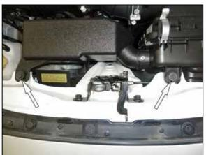
6. Remove the two bolts shown securing the resonator and air box to the core support. **NOTE: These bolts will be reused in a later step.**
