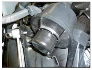
21. Install the provided caplug onto the sound
