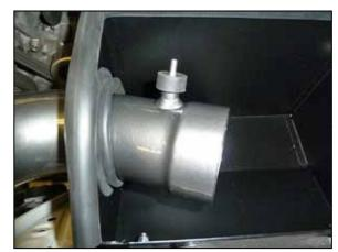
18. Install the tube through the heat shield and then install the provided rubber mounted stud onto the tube as shown.
