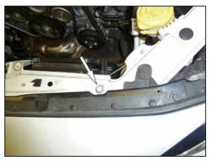
15. Remove the core support bolt shown. **NOTE: This bolt will be reused.**
