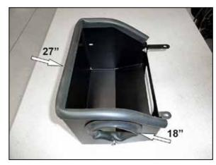
14. Install the 13" long section of edge trim into the hole of the heat shield as shown and then install the 27" long section of edge trim onto the top of the heat shield as shown.
