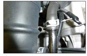
3. Release the spring clamp and then disconnect the crank case vent hose from the fitting.
