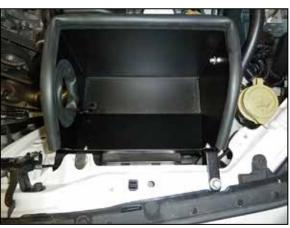
16. Set the heat shield into position on the core support and secure with the factory air box mounting bolts and to the previously installed bracket with the hardware provided.
