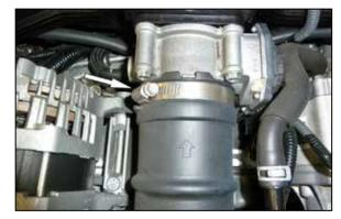
4. Loosen the hose clamp securing the intake hose to the throttle body.
