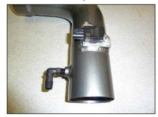
17. Remove the mass air sensor from the factory air filter housing and then install it into the AEM® intake tube using the provided hardware. Install the provided 90° vent fitting into the AEM® intake tube as shown.
