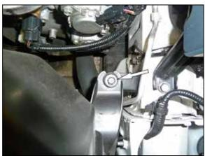
7. Remove the remaining air box mounting bolt then lift up the air box assembly and remove it from the vehicle.
