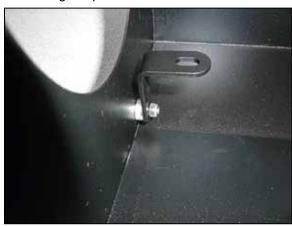
12. Install the provided "L" bracket (070015) onto the heat shield using the provided spacer between the bracket and heat shield and hardware.
