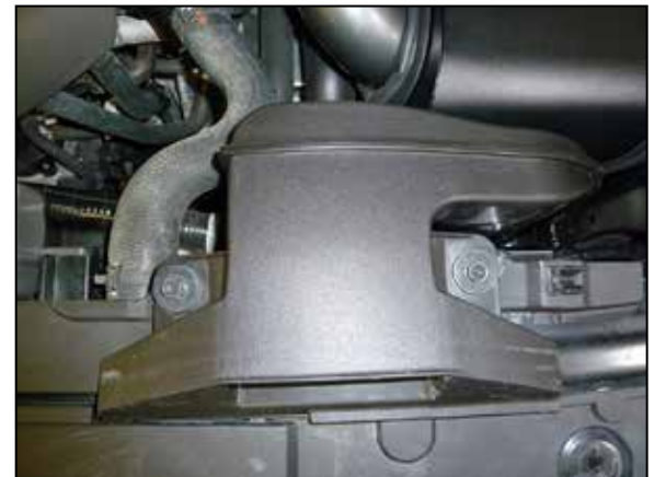
20. Install the factory fresh air scoop bolts.
