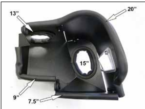
11. Install the cut edge trim onto the heat shield as shown.
