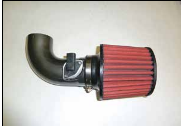
14. Install the AEM® air filter onto the AEM® intake tube and secure with the provided hose clamp.
