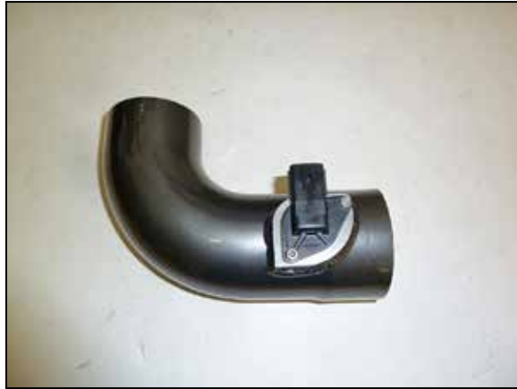
13. Remove the mass air sensor from the factory air filter housing and install it into the AEM® intake tube and secure with the provided hardware.
