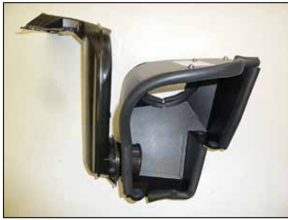
12. Install the factory fresh air intake scoop into the AEM® heat shield as shown.
