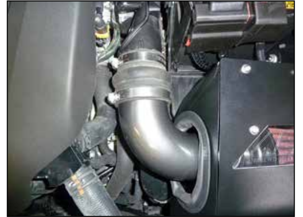
19. Install the intake tube into the coupler hose, adjust the tube for best fit and then secure the hose clamp.
