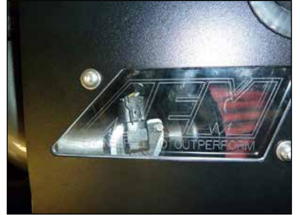
18. Reconnect the mass air sensor electrical connection.
