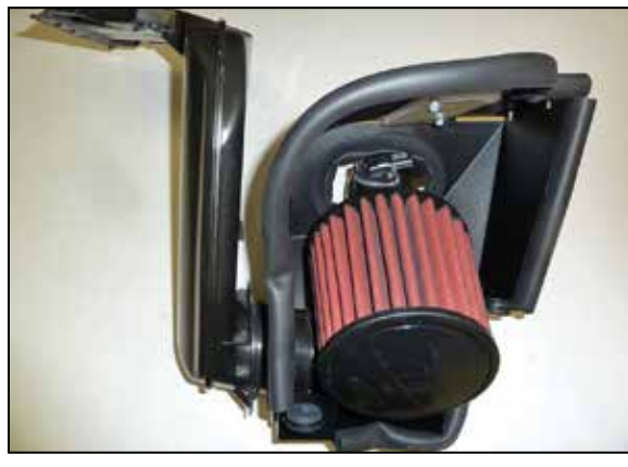
15. Install the intake tube assembly through the hole in the heat shield as shown.
