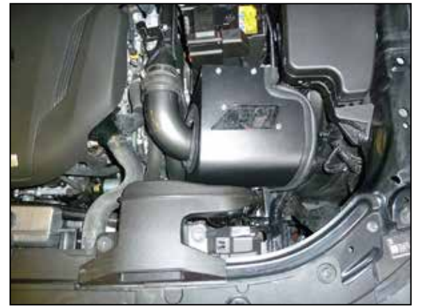
17. Install the AEM® intake assembly into the vehicle so the mounting grommets secure over the factory mounting studs.
