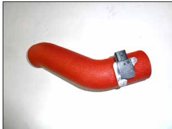
12. Remove the mass air sensor from factory housing and install it into the AEM® tube using the provided hardware.
