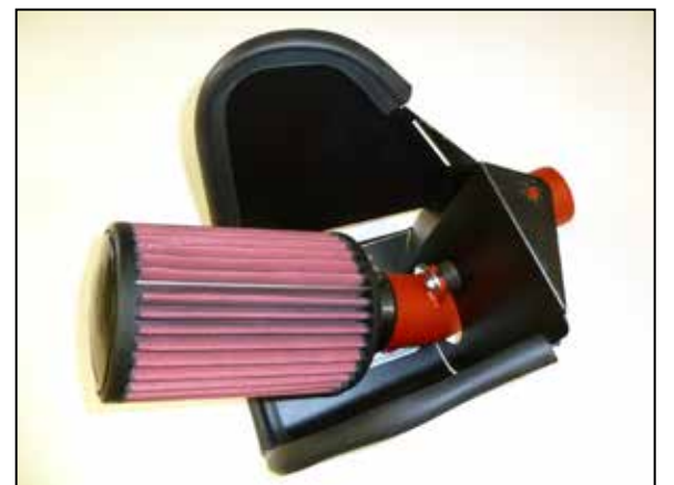
15. Install the AEM® air filter onto the intake tube and secure with the provided hose clamp.
