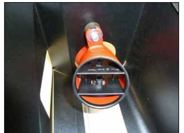
14. Install the intake tube through the heatshield and secure with the provided rubber mounted stud and hardware.
