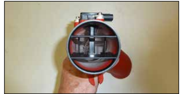
13. Place three small drops of the provided glue next to the lip of the maf sleeve and then install the maf sleeve so that the blades are perpendicular to the maf as shown.
