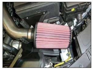
15. Install the AEM<sup>®</sup> air filter onto the intake tube and secure with the provided hose clamp.
