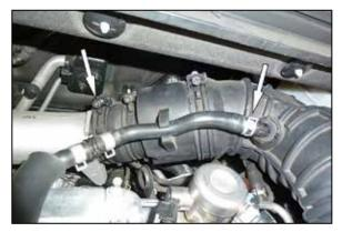
3. Loosen the clamp that secures the factory intake tube to the turbo inlet pipe. Release the spring clamp that secures the PCV hose to the intake tube and then disconnect the PCV hose.
