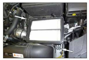
7. Remove the three bolts that secure the lower air filter housing and then remove the lower housing and fresh air duct from the vehicle. NOTE: AEM recommends that customers do not discard factory air intake.
