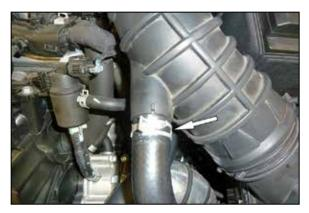
4. Release the spring clamp that secures the BOV hose to the intake tube and then disconnect the BOV hose.
