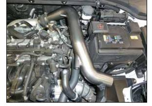
13. Install the intake tube into the coupler and onto the heat shield, adjust for best fit and then secure with the provided hardware.
