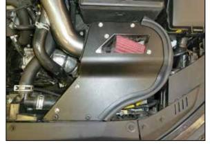
18. Install the heat shield lid and secure with the provided hardware.
