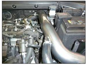
14. Connect the PCV hose and BOV hose to the AEM<sup>®</sup> intake tube and secure with the factory spring clamps.
