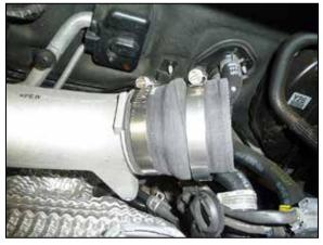
12. Install the provided coupler (08439) onto the turbo inlet and secure with the provided hose clamp.
