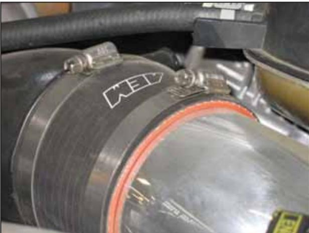
i. Install the intake pipe into the coupler on the turbo inlet. Align the intake pipe mounting bracket with the previously installed aluminum stand. Use a #64 hose clamp to secure.
