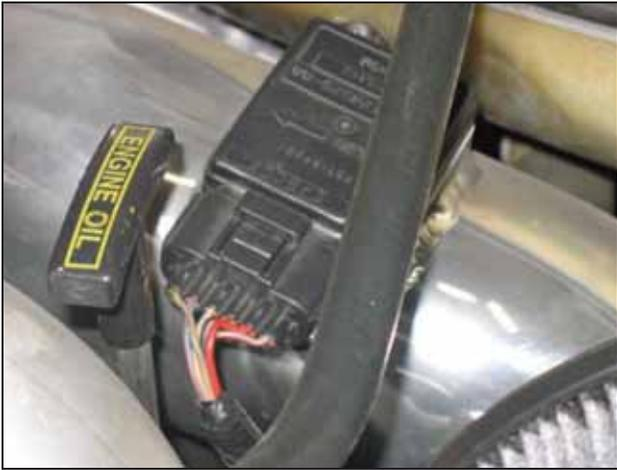
o. Depending on application, connect the wiring harness plug into the MAF or IAT sensor. Rotate the oil dipstick to allow sufficient clearance.
