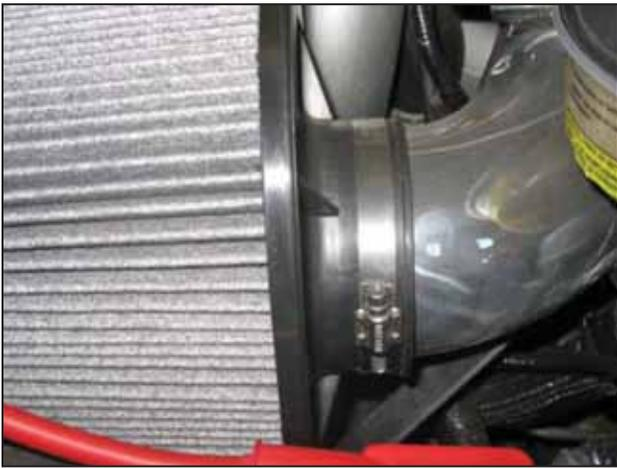
m. Slide the hose clamp onto the air filter's neck and attach the air filter assembly onto the filter adapter. Ensure the air filter is completely seated onto the adapter and the hose clamp is aligned with the filter adapter's lip. Once the hose clamp is properly aligned, secure the hose clamp, ensuring the filter neck's tabs compress and engage.
