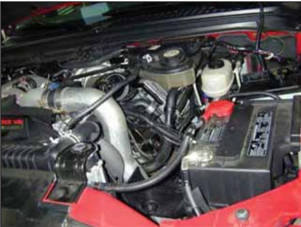
c. Factory air box system removed.
