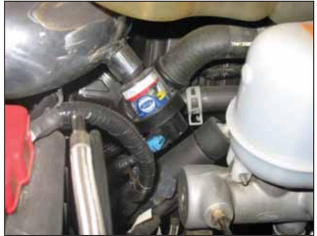
p. Plug the air filter restriction gauge into the wiring harness. Ensure the wiring harness will not make contact with any components that will get HOT.
