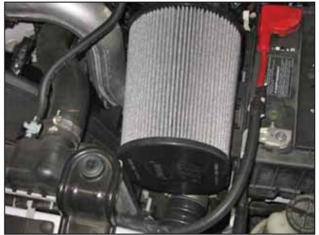
n. Ensure the air filter does not make contact with any part of the vehicle and has adequate clearance.
