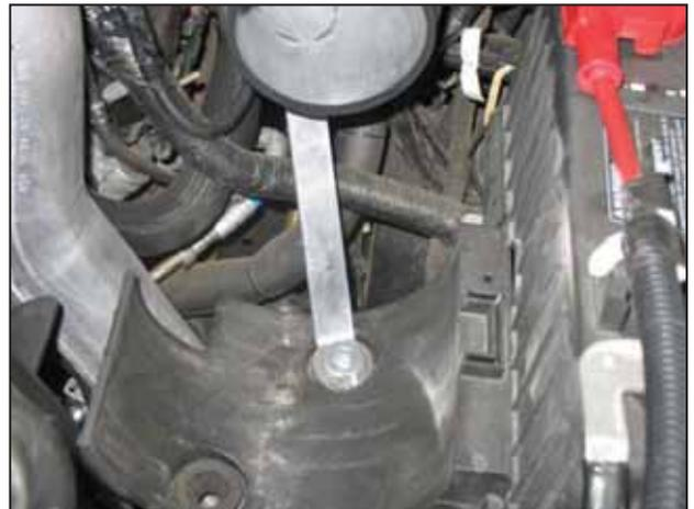
j. Install the supplied M6 washer and bolt through the bottom of the aluminum stand. Secure the bolt using another M6 washer and serrated nut as illustrated in step 3k.
