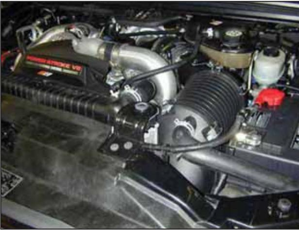
a. Stock intake system. Unplug the wiring harness from the inlet air temperature (IAT) sensor or mass air flow (MAF) sensor. All vehicles have one or the other.
