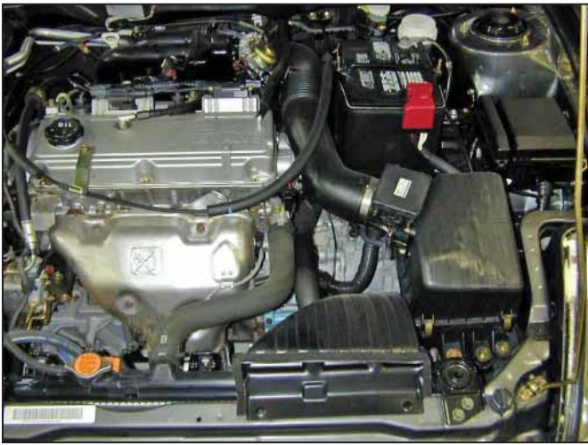
a. Factory air box system installed.
