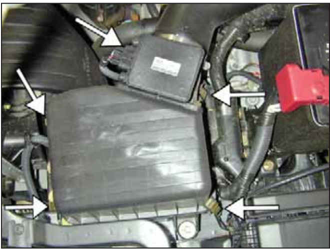
c. Unplug the MAF sensor. Remove stock inlet pipe. Release four clamps on the air box and remove upper air box from the vehicle.
