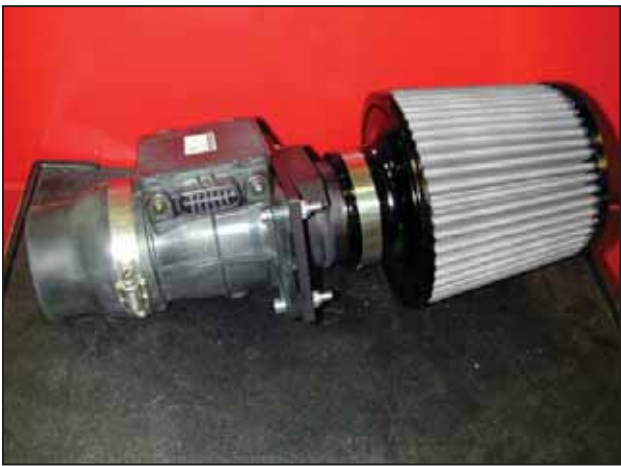
h. Install the air filter on to the MAF sensor adapter. Tighten the air filter hose clamp.
