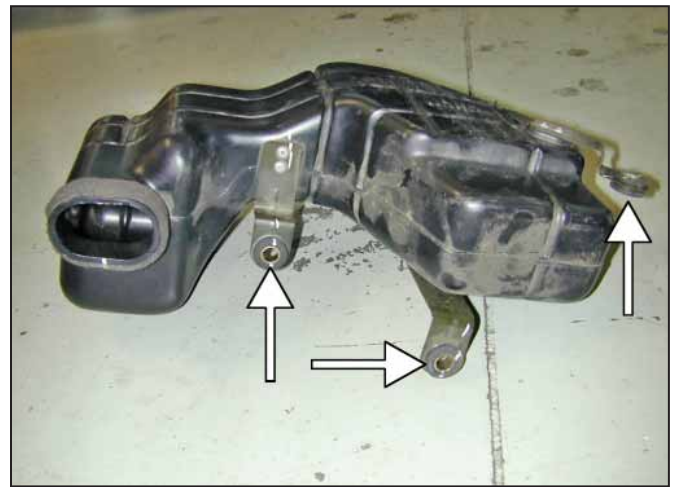
h. Loosen the three bolts that hold in the lower air box and remove it from the vehicle.
