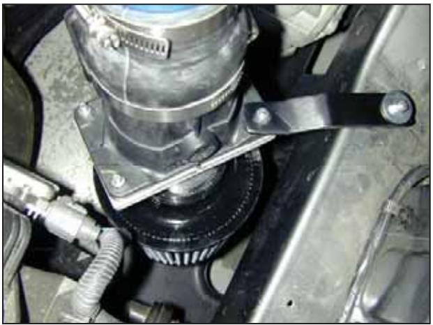
i. Install the MAF sensor assembly to the inlet pipe with a hose clamp. Attach support bracket as shown (See diagram for proper installation). Do not completely tighten the lock nut. Plug in the MAF sensor.
