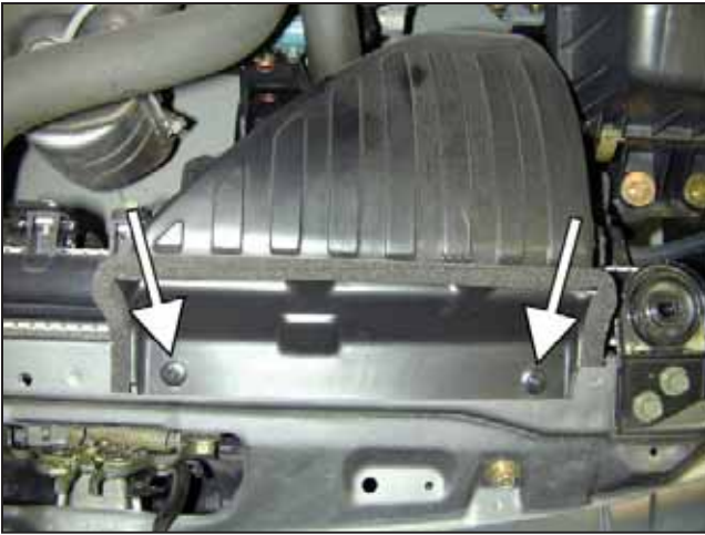
e. Release air snorkel by first pressing in the centers of the plastic rivets.
