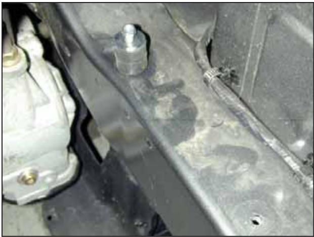
g. Install rubber mount in threaded hole as shown.
