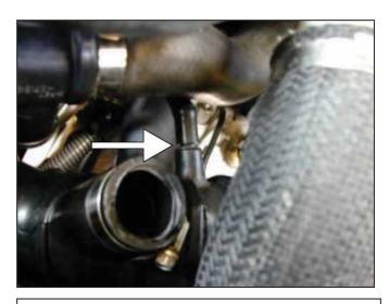
j. Disconnect the crankcase breather tube at the turbo inlet hose.
