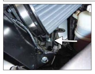
o. Attach the air filter and MAF sensor assembly to the inlet pipe. Line up the bracket to the rubber mount. Refer to the diagram on the next page.
