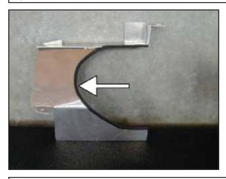
q. Attach the rubber edge trim to the heat shield.
