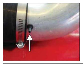
e. Insert vacuum adapter into the rubber grommet.
