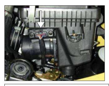
f. Disconnect the MAF sensor harness from the bottom portion of the air box. Carefully remove the bottom portion of the air box. The honeycombs in the MAF sensor are sensitive, take note not to damage during removal.
