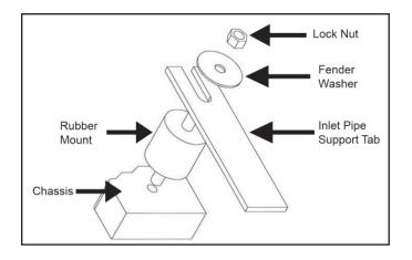
Proper rubber mount installation.
