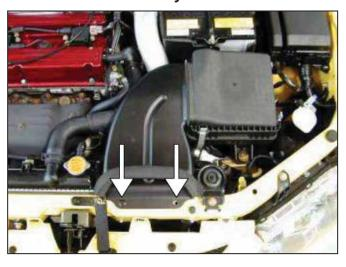
a. Push in the inner circle on the clips to remove them. Remove both clips. Remove inlet duct to air box.
