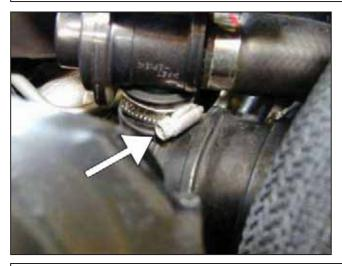
h. Loosen the hose clamp connecting the blow off valve to the turbo inlet hose. Disconnect the blow off valve from the inlet hose. Remove hose clamp from the inlet hose.
