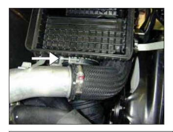
e. Loosen the hose clamp connected to the bottom portion of the air box.
