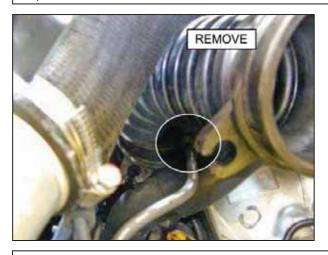
k. Disconnect vacuum line from the boost solenoid to the turbo inlet hose. The vacuum line is located underneath the turbo inlet hose. Remove the turbo inlet hose.
