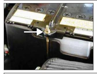
p. Unbolt nut to the battery bracket.
