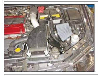
s. Re-attach the factory inlet scoop and secure with the original push-in tabs.
