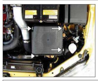
c. Unfasten the 4 clips that hold down the top to the air box. Remove the air box top.
