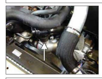
g. Insert BOV outlet into the BOV hose. Make sure you rotate the BOV toward the firewall, so that it clears the coolant hose.
