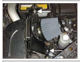
r. Insert heat shield. Alsign with the battery bracket and secure with a washer and factory nut. Secure the other mounting point of the heat shield with the provided bolt.
