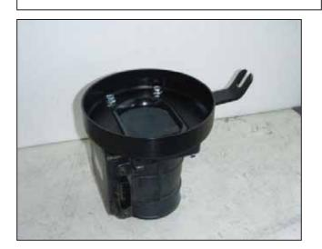
I. Assemble the MAF sensor adapter to the MAF sensor with the provided M6 nuts and M6 bolts.
