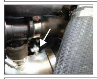
i. Secure the factory breather hose to the nipple with the provided hose clamp.
