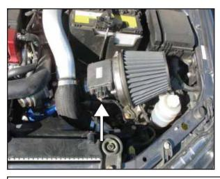
p. Reattach MAF sensor harness. Some vehicles may require that you remove approximately 2" of wire loom tape to create more slack to route the MAF harness.
