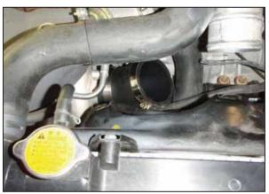
c. Attached assembled coupler to the turbo inlet as shown.
