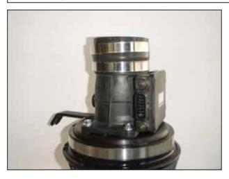
n. Attach the coupler to the MAF sensor. Attach the provided hose clamps to the coupler as shown. Do not fully tighten. You may need to add a very small amount of lubricant to slide the coupler over the sensor for easier installation.
