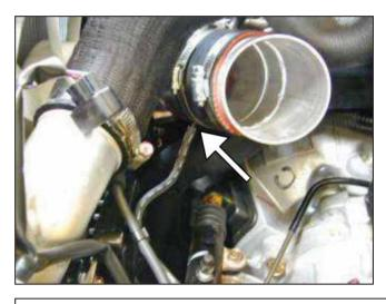
k. Attach vacuum line from the boost solenoid to the vacuum nipple underside of the pipe.
