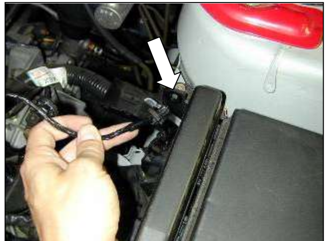
j. Unclip the MAF sensor wiring harness from the bracket on the shock tower.
