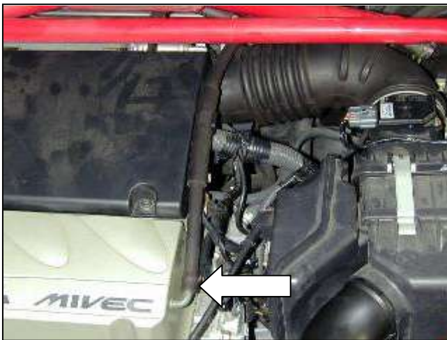
c. Remove the breather hose from the valve cover.
