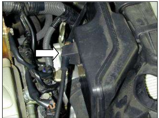
d. Unclip the throttle cable from the side of the air filter housing.
