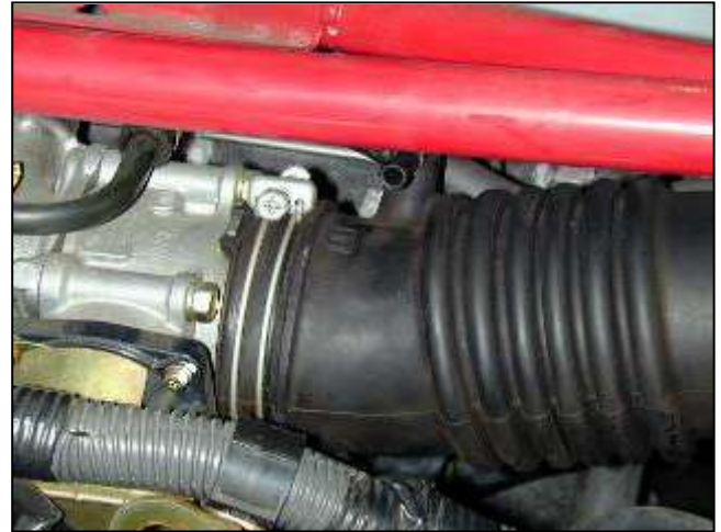
f. Unscrew the inlet tube clamp and remove the inlet tube from the throttle body.
