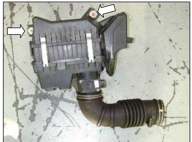
h. Remove the two bolts securing the stock air filter housing to the engine bay. Remove the air filter housing and the inlet tube from the vehicle.
