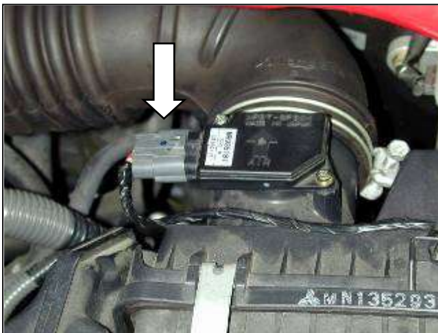
g. Unplug the MAF sensor harness connector.
