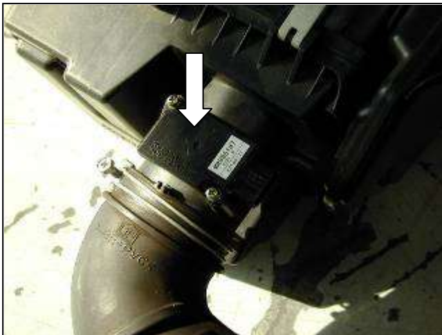
i. Remove the two bolts securing the MAF sensor to the air filter housing; remove the MAF sensor. Be careful not to damage the sensor.
