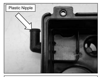
j. Remove the plastic nipple from the lower air cleaner housing and set aside as it will be used with the installation of the AEM<sup>®</sup> intake.
