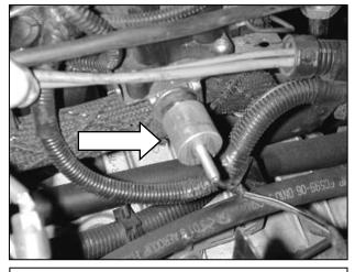
d. Remove the distributor coil pack bracket bolt and replace with the supplied stud and standoff.
