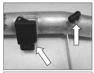
c. Install the mass air flow sensor and the plastic nipple onto the  $\text{AEM}^{\$}$  intake pipe.
