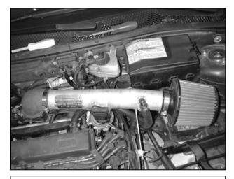
AEM<sup>®</sup> intake system installed
