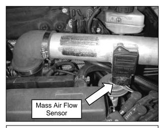
g. Install the supplied breather hose onto the valve cover nipple and secure with a 1" hose clamp. Also connect the wiring harness connector to the mass air flow sensor.
