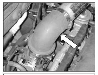
e. Install the supplied rubber elbow on the throttle body using the supplied 3" hose clamp. Install the intake pipe into the rubber elbow and secure it with the supplied 2.5" hose clamp.
