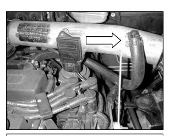
h. Install the second end of the breather hose onto the plastic nipple as shown. Secure with the supplied 1" hose clamp.
