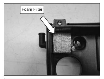
i. Remove the foam filter from the lower air cleaner housing.
