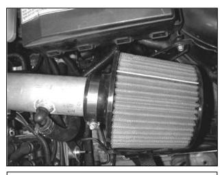
i. Install the AEM<sup>®</sup> air filter onto the intake pipe and secure with the supplied hose clamp.
