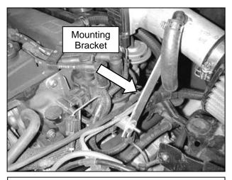
f. Line up the intake pipe mounting bracket with the stud and standoff and secure with the supplied washer and lock nut.
