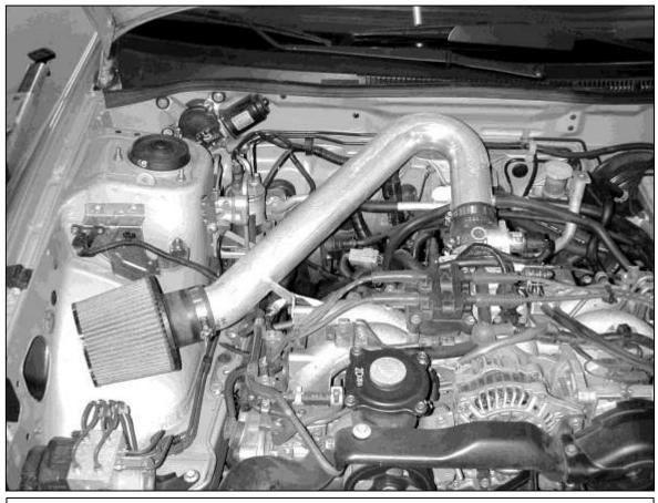
AEM<sup>®</sup> intake system installed
