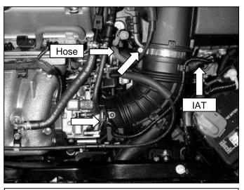
b. Loosen the two clamps securing the inlet tube to the throttle body and air cleaner. Unplug the intake air temp sensor and unplug the hose going to the inlet tube. Remove the inlet tube from the vehicle
