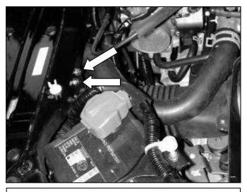
e. Loosen the two nuts securing the air tube, then remove it.
