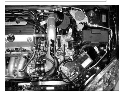
e. Install the intake pipe assembly, placing the reducer coupler over the throttle body. Also secure the bracket over the aluminum spacer with the included washer and serrated nut. Install the factory breather hoses over the nipples on the intake pipe.
