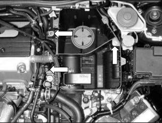
d. Loosen the 3 bolts holding the air filter assembly, and remove it.
