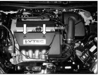
a. Loosen the two bolts holding the intake cover, then remove it.
