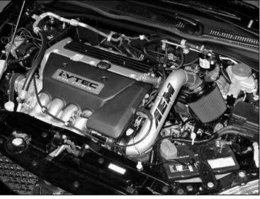
f. Install the intake cover, using the original bolts. Plug the IAT wiring harness back into the IAT sensor.
