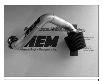
d. Install the air filter and reducer coupler onto the intake pipe using the supplied hose clamps, as shown.
