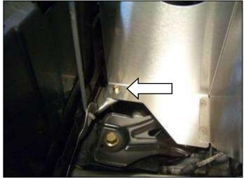
g. Secure the heat shield with the bolt removed in step 2i.
