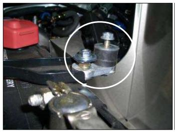
h. Attach the rubber mount assembly to the battery bracket. Secure with the original nut. Secure the heat shield with provided washer and nylok nut.
