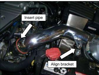
i. Insert the inlet pipe into the coupler. Align the inlet pipe with the rubber mount.
