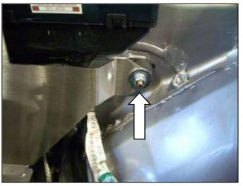
f. Insert the heat shield and attach to open rubber mount from step 3d. Attach a fender washer and nylok nut, tighten.
