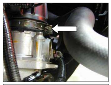
a. Loosen the hose clamp at the throttle body that secures the inlet tube.
