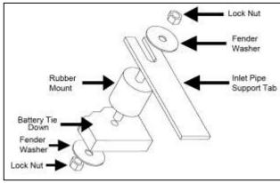
o. Secure inlet pipe to the rubber mount. Attach the air filter and secure.
