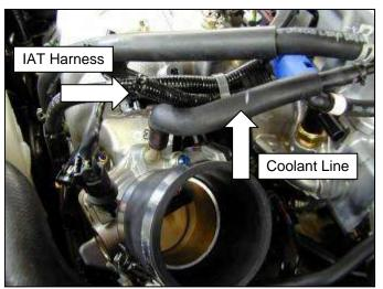
b. Make sure the IAT sensor wiring harness is above the coolant line.
