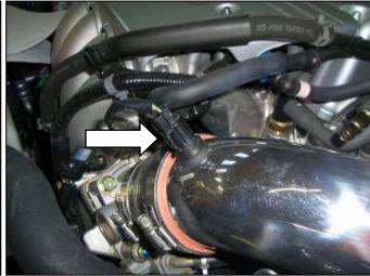
k. Insert Inlet Air Temperature (IAT) sensor.
