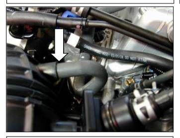
c. Remove breather hose from the inlet air tube
