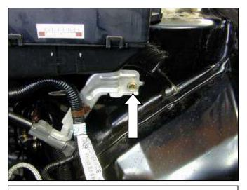
i. Remove bracket bolt. This bolt will be reused in the installation.
