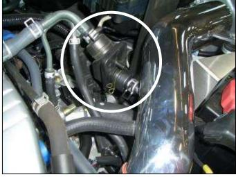
n. Attach the oil trap coupler to the oil trap and secure with the clamp from step 3m. Secure the oil trap coupler to the angled nipple on the inlet pipe with provided spring clamp.
