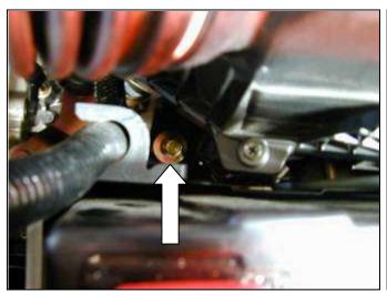
g. Loosen and remove the bottom bolt to the air box. Remove inlet air tube and air box assembly.
