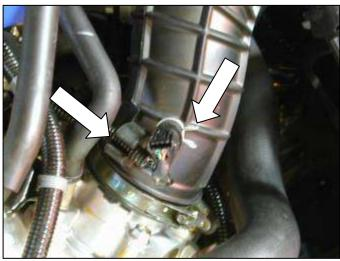
b. Squeeze the clamp holding the Inlet Air Temperature (IAT) sensor. Remove IAT sensor from inlet air tube. Remove wiring harness from the inlet air tube.
