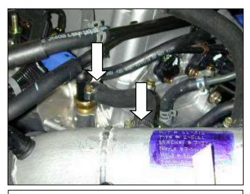
I. Attach breather hose to the crankcase and to the nipple perpendicular to the inlet pipe. Secure with hose clamps. Make sure the hose does not kink.
