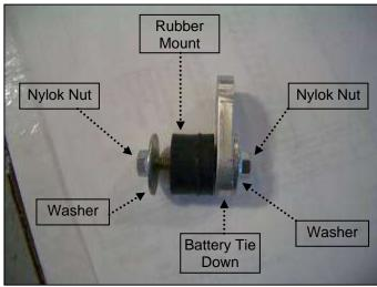
e. Assemble second rubber mount, 5/8". On one end attach fender washer and nylok nut, do not tighten. On the other end, attach the battery tie down, fender washer, nylok nut and then tighten hardware.
