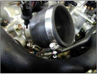
c. Attach reducer coupler with hose clamps as shown. Use the #44 hose clamp on the throttle body side and the #48 on the opposing side.
