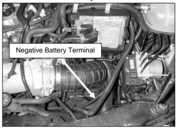
a. Locate the negative battery terminal and disconnect.
