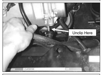
i. Unclip the idle air hose from the throttle body. Remove the four bolts securing the throttle body to the intake manifold.
