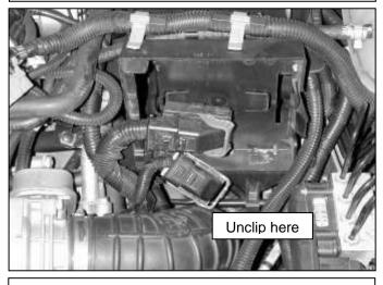
c. Remove the ECU from the housing by unclipping it on the driver's side.
