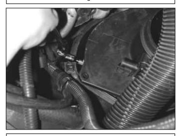
d. This step is complicated so take your time. Using a 90 degree pick, slide the pick into the hole on the top of the housing and under the lip on the filter. Pull up on the filter until it is all the way on the air box inlet tube. **Be careful not to damage the MAF sensor.** Tighten the hose clamp on the filter by lifting up on the air box lid as shown.
