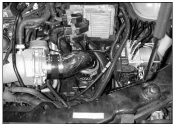
AEM® intake system installed
