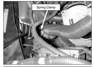
e. If step 3c is too complicated or you do not have the proper tools, the radiator hose can be removed to install the air filter and air box lid.
