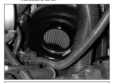
b. Check to be sure the AEM<sup>®</sup> air filter is free from any foreign objects. Set the air filter in the stock air filter housing. Be sure to angle the hose clamp towards the center of the grill as shown.
