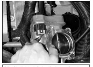
j. Unplug the throttle body wiring harness from the bottom side of the throttle body.
