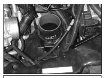
g. Reinstall the three screws to secure the air box lid. Install the reducing couple onto the air box outlet tube. Secure the coupler using a #52 hose clamp as shown.
