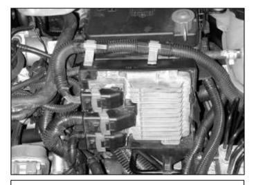
b. Disconnect the main harness from the ECU. This is done by releasing the lock down and pulling on the wire side of the 3 plugs.
