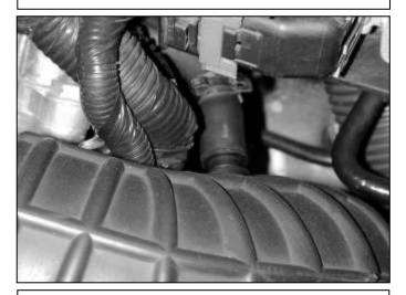
d. Using pliers, remove the retaining clamp from the breather hose attached to the air inlet tube. Disconnect the breather hose from the inlet tube.
