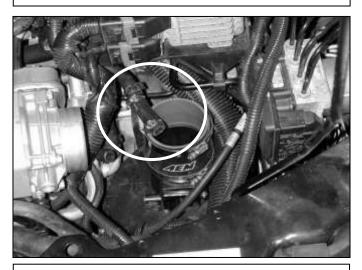
h. Using the supplied ½" hose, attach the hose to the stock plastic barb fitting. Secure using the supplied ¾" hose clamps.
