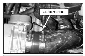
k. Reinstall the ECU and reconnect the harness. Use the supplied zip tie to secure harness wires as shown.
