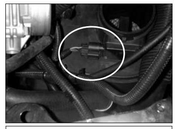
f. Unclip the Mass Air Flow (MAF) sesnor wiring harness from the sensor.
