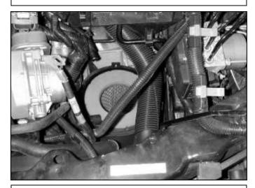
h. Remove the stock air filter from the air filter housing.
