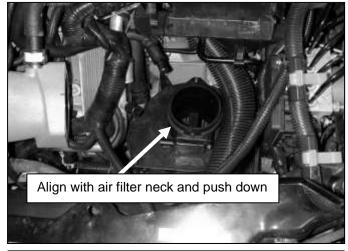
c. Install the air box lid by sliding it under the radiator hose and aligning the air box inlet tube with the air filter neck. Push down on the air box lid once it is aligned.
