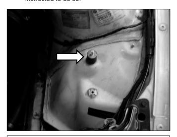
b. Insert the rubber mount as shown.
