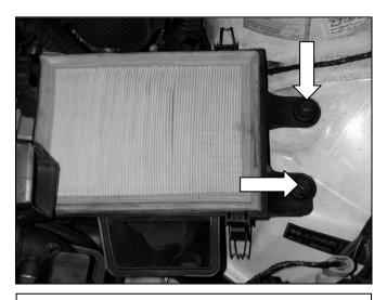
e. Loosen and remove the 2 bolts holding the bottom of the air box. Remove the air filter element and the lower half of the air box.
