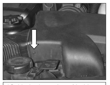
d. Push in tab and remove the top of the air box.
