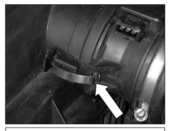
c. There are 2 clips holding the air box to the MAF sensor.
