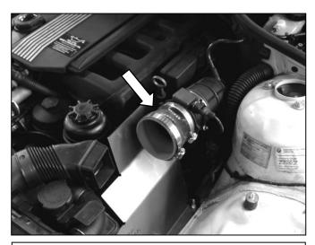
e. Attach the coupler and hose clamps to the MAF sensor as shown.
