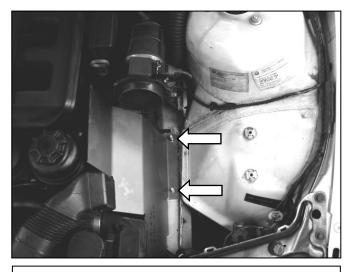
d. Insert the heat shield. Secure with washers and nylok nuts.
