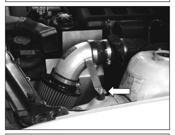
f. Attach the air filter to the inlet pipe. Then attach the assembly to the coupler that was installed on the MAF sensor in step 3e. Align the intake bracket with the rubber mount stud and secure with a washer and nylock nut. Refer to the diagram for proper installation. Ensure the air filter and intake pipe have adequate clearance. Once proper fitment is achieved secure all hardware.
