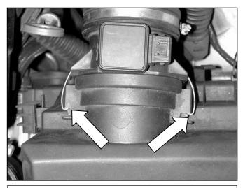
b. Unfasten both clips holding the air box to the MAF sensor.
