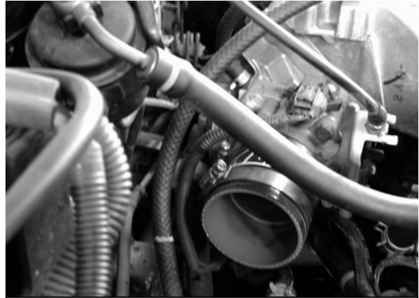
b) Insert the 2.75" silicone coupler on to the throttle body. Place two #44 hose clamps on the coupler but do not tighten yet.
