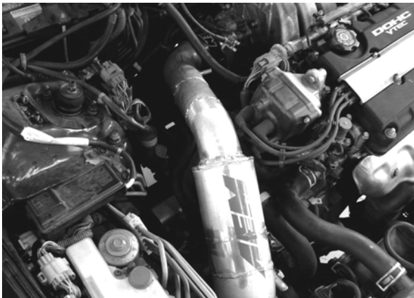
c) Insert the AEM intake pipe in to the engine bay with the 2.75" end at the throttle body. Slip the end of the pipe in to the silicone coupler.
