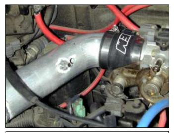
d. Ensure that the inside of the AEM<sup>®</sup> inlet pipe and air filter are clean and free from any foreign objects and/or obstructions. Slip the intake pipe under the cables and insert the small end of the intake pipe into the hose on the throttle body. The throttle body end is the end with the breather hose nipple.
