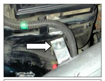
g. Slide the inlet pipe support over the rubber mount. Use the supplied washer and lock nut and assemble as shown. Next install the AEM<sup>®</sup> air filter on to the end of the intake pipe. Push the air filter over the intake pipe until it mates to the step inside of the filter inlet. Install the supplied hose clamp to secure the air filter onto the inlet pipe. Tighten the hose clamp after this is done.
