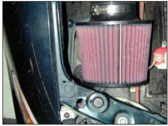
h. Ensure that the air filter is not touching any part of the vehicle. Position the inlet pipe for best fitment. Be sure that the intake pipe and any of its components do not make contact with the vehicle. Tighten the hose clamps at the throttle body. Tighten the bolt on the rubber mount. Check for proper hood clearance. Re-adjust the intake pipe if necessary.
