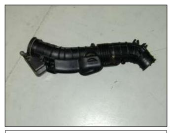
i. Remove the connecting hose and air chamber as one piece.
