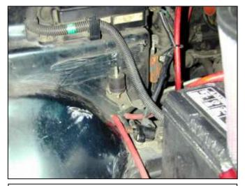
e. Thread the supplied rubber mount into the tab where the original air filter box was located. This tab is located on the front side of the strut tower.
