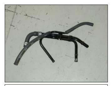
c. CAUTION: Ensure the engine is completely cool before removing the coolant hose, or hot coolant will escape from the cooling system and cause injury or damage. Be sure to capture any lost coolant in a clean container.
