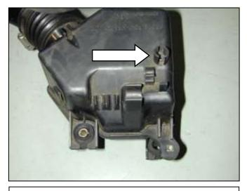
h. Unplug the two breather hoses that attached the tube connecting the air filter housing to the throttle body. Loosen the hose clamp on the throttle body and slide the tube out and up. Be sure to disconnect the vacuum lines connected to the air chamber under the main tube.
