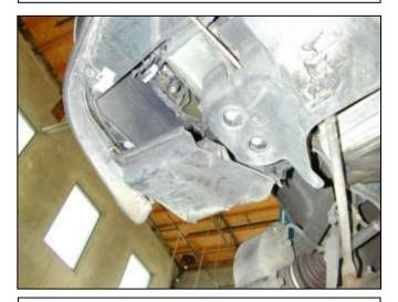
d. Raise the front of the vehicle with a jack. Refer to your owner's manual for proper jack and jack stand placement to properly support vehicle. Support your vehicle using properly rated jack stands before wheel removal or while working under the vehicle. **NEVER WORK UNDER A VEHICLE WITHOUT USING JACK STANDS.**
