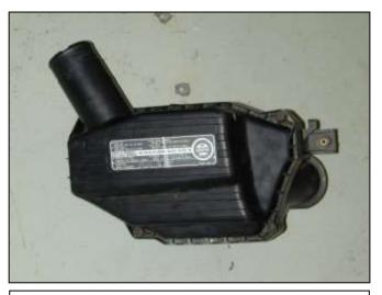
g. Unscrew the two bolts securing the air filter housing and pull the housing out of the car.
