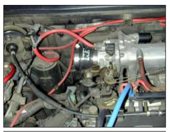
c. Install the 2.5" coupler on the throttle body using both 2.5" hose clamps.
