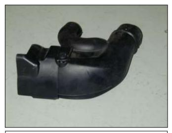
f. Remove the intake air duct in front of the air filter housing by simply pulling up on it.
