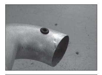
f. Install the supplied rubber grommet and IAT sensor into the AEM® intake pipe.
