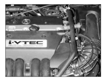
b. Make note there is one breather hose, one vacuum hose, and one intake air temperature (IAT) sensor.
