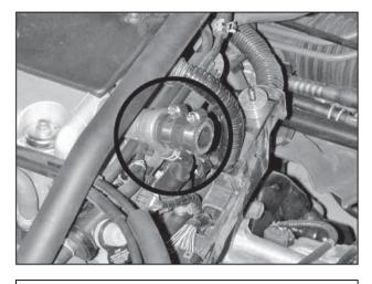
d. Replace the factory breather hose with the supplied breather hose. Use the supplied 1 1/4" hose clamps to secure the breather hose in place.
