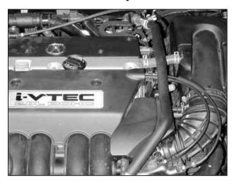
a. Remove the two mounting bolts securing the upper engine cover. Remove the engine cover.
