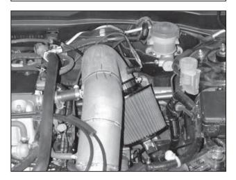
AEM® intake system installed
