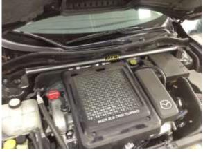
a. . Place the AEM Strut Tower Bar over strut tops, and replace the strut top bolts.
