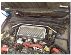
a. Install the AEM Strut Tower Bar, replace the original strut tower nuts, and tighten.
