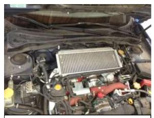
a. Remove the 4 Strut Tower nuts needed to install the AEM Strut Tower bar.
