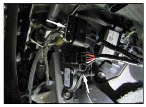
3. Connect the pedal module wiring harness into the pedal assembly and then connect the factory wiring harness into the pedal module wiring harness.
