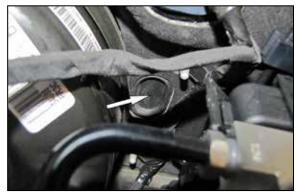
11. Poke a small hole in the existing firewall grommet and feed the boost control knob wiring harness through the grommet from the inside of the vehicle. Connect the control knob wiring harness to the pigtail connected to the module. And secure with the provided tie wraps. **NOTE: be sure the wiring harness is routed in such a way that in it is not near any moving components or heat sources.**
