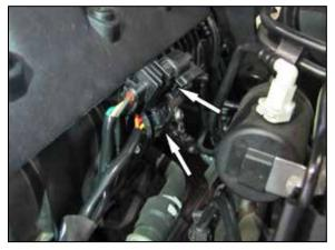
8. Connect the K&N<sup>®</sup> wiring harness to the MAP sensor and to the factory wiring harness.
