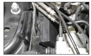
10. Mount the boost module in a suitable location such as on the back side of the shock tower as shown and secure with the provided tie wraps.
