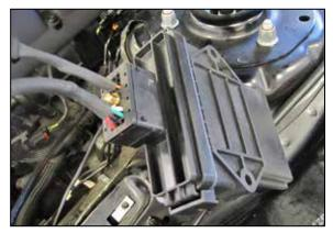
9. Route the K&N<sup>®</sup> wiring harness towards the driver's side inner fender and connect it to the boost module.
