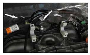
4. Connect the K&N® wiring harness to the MAP sensor and to the factory wiring harness. Route the K&N® wiring harness towards the driver's side inner fender. Secure the wiring harness with the provided tie wraps. Reinstall the decorative engine cover.
