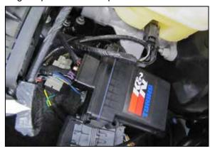
6. Connect the boost module wiring harness to the module and secure with the locking bolt.
