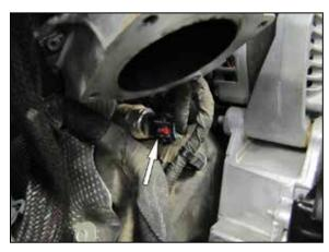
7. Locate the Fuel rail pressure sensor under the charge manifold. Release the locking tab and disconnect the factory wiring harness from the sensor.
