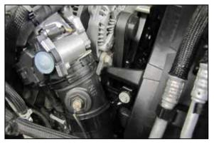
10. Reconnect the charge tube to the throttle body, be sure the locking ring has the charge tube locked onto the throttle body. Reinstall the charge tube mounting bolt.
