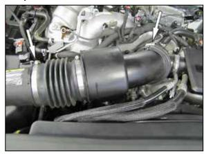
2. Loosen the hose clamps that secure the intake tube and then remove the intake tube from the vehicle.
