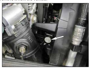
4. Remove the intake charge pipe mounting bracket bolt.
