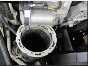
5. Release the charge pipe locking ring by rotating it clockwise and pulling the tube down away from the throttle body.
