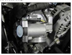
6. Disconnect the throttle body electrical connection and then remove the four bolts that secure the throttle body to the charge manifold. Remove the throttle body and gasket from the engine.
