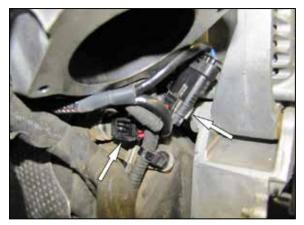
8. Connect the provided Boost module wiring harness to the factory wiring harness and to the fuel pressure sensor.
