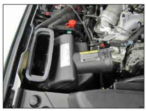
3. Lift the air filter housing assembly up and remove it from the vehicle.
