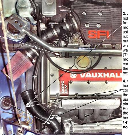
**3.** Attach the large 2 holed washer to the front air box mounting point using the original rubber mounting, nuts, 6mm spring washers and flat washer supplied. (The original rubber mounting bobbin can be located on the front of the air box.
