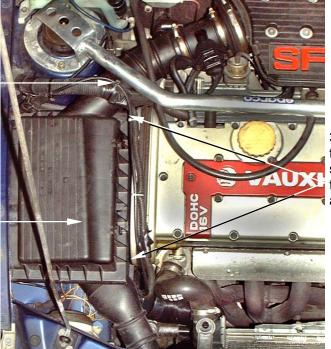
**3.** Remove the nuts from the rubber mountings securing the air box base to the chassis leg, lift out the air box base assembly.
