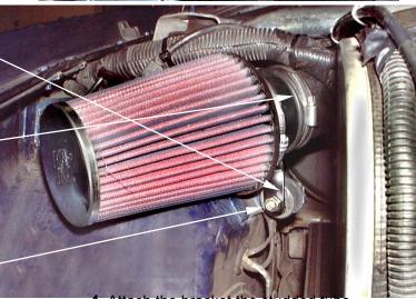
4. Attach the bracket the studded tube using the nuts and washers supplied.
