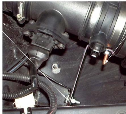
2. Fit the studded clip to the intake hose, do not tighten the clip yet. Attach the studded clip to the mounting bracket and secure with a nut and washers supplied.
