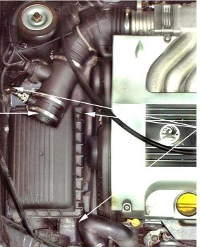
**3.** Remove the 3 securing nuts from the air box base and lift out the complete assembly
