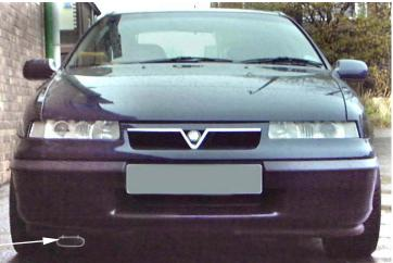
Pierce / drill two 3mm holes in the front bumper trim, secure to the front bumper using 2 plastic ties. Insert the flexi cold scoop, secure the scoop to a hole in the cross member with
