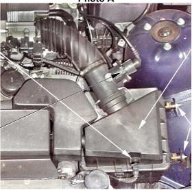
**3.** Unclip and remove the air box lid from the air box base.
