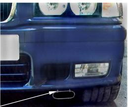
Taking all of the necessary safety precautions as per the manufacturers instructions carefully raise the front of the car. Unclip and remove the under tray side trim. Once the trim has been removed, refit the 2 securing screws to the under tray / wheel arch liner. Pierce drill two 3 mm holes in the front lower spoiler trim and secure the new cold air scoop to it using a long plastic tie. Secure the rear of the scoop to the wheel arch liner.
