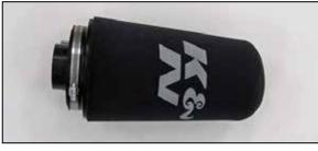
14a. Install the provided foam wrap onto the  $K\&N^{\ensuremath{\circledast}}$  air filter.
