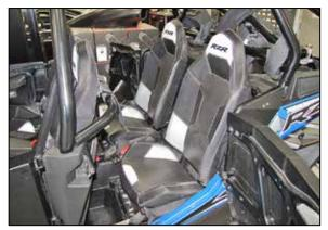
2. Release the locking leaver and remove the (rear) seats from the vehicle and set aside. Remove the eight bolts shown that secure the rear panels. NOTE: Six of these bolts will be reused in a later step.
