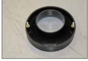
13. Install the two provided 6mm studs into the radius filter adapter as shown.
