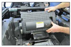
6. Remove the air filter housing from the vehicle. NOTE: K&N Engineering, Inc., recommends that customers do not discard factory air intake.
