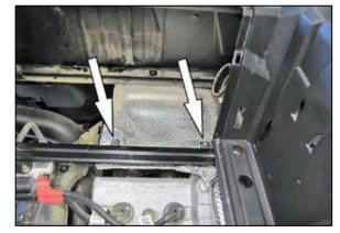
9. Remove the two nuts and bolts shown that secure the heat shielding to the chassis.
