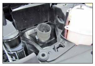
28. Install the fresh air intake hose (08429) onto the Fresh air intake tube. Adjust the tube so that it is tight against the housing, slide the hose down tight against the housing and then secure the hose clamp.
