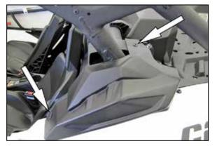
2. Remove the two fasteners securing the corner cap and then remove the corner cap from the vehicle.
