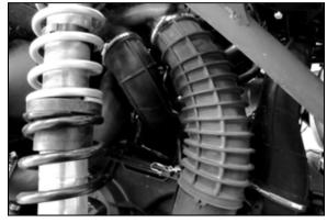
30. Reinstall the clutch fresh air intake hose and secure with the factory hose clamp.
