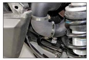
27. Install the 90° fresh air hose (084102) onto the air filter housing inlet and then onto the fresh air intake tube. Then secure with the provide hose clamps.
