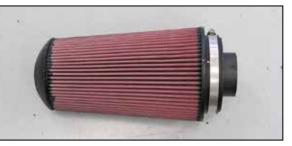
21. Install the filter adapter into the K&N<sup>®</sup> air filter and secure with the provided hose clamp.
