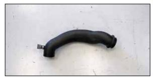
25. Install the duck bill onto the fresh air intake tube and secure with the provided hose clamp.
