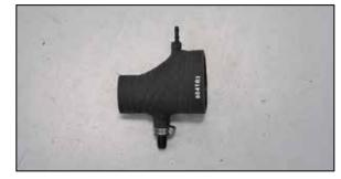
19. Install the two provided vent fittings into the K&N<sup>®</sup> intake hose (084103) and secure the large fitting with the provided hose clamp.
