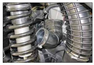
14. Loosen the hose clamp securing the clutch intake hose and disconnect the hose and set aside for access to the air filter assembly.
