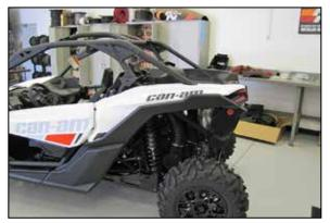
34. Reinstall the fender and corner cover and secure with the factory hardware and clips.
