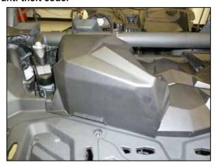
2. Remove the factory intake dust cover by pulling upwards to dislodge it from the mounting grommets.
