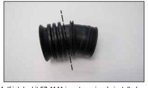
4. If intake kit 57-1141 is not previously installed, remove the factory bellows from the vehicle and trim it where indicated and then reinstall the bellows.
