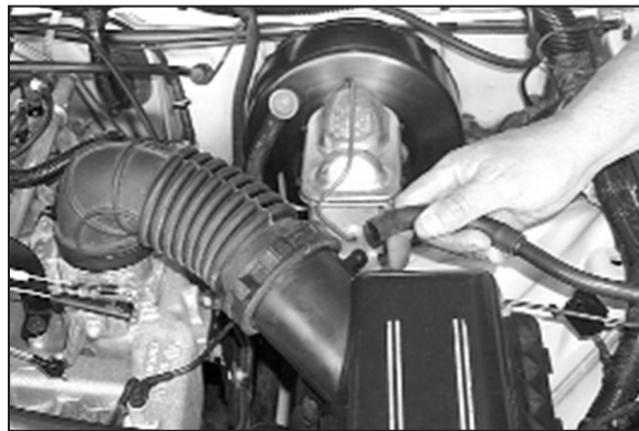
3. Remove the EVAP canister vent line from the air cleaner lid
