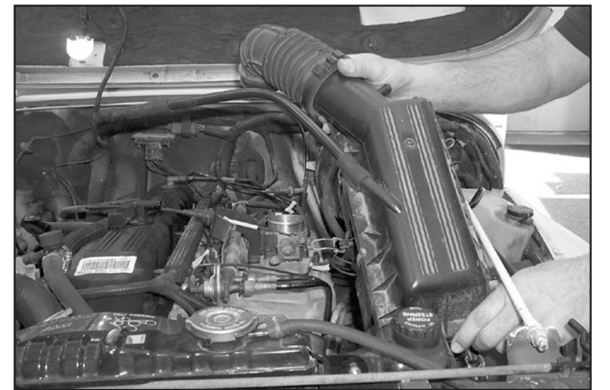
5. Unclip the three lower air cleaner retaining clamps, then remove the upper air cleaner assembly as shown.
