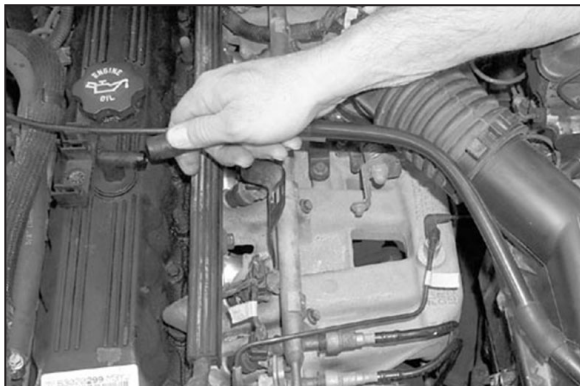
2. Disconnect the crank case vent hose.
