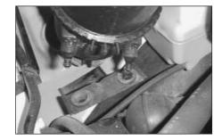
6. Pull firmly up on airbox to release airbox from grommets on lower airbox support bracket assembly.
