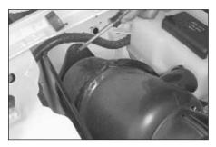
3. Using a flat blade screwdriver, remove the push clip.
