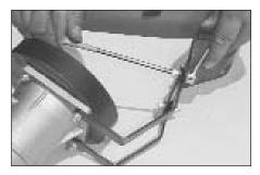
13. Using the hardware and support brackets provided, attach the mass air assembly to the airbox support bracket.
