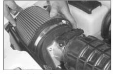
17. Install the air filter element onto mass air adapter and secure with the provided hose clamp.
