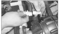
Reconnect the secondary mass air sensor electrical connection.
