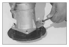
9. Loosen and remove the nuts from the mass air sensor. NOTE: It may be necessary to use vise grips to secure studs. 12. Using the hardware provided, assemble the mass air adapter, gasket and brackets as shown in illustration above.
