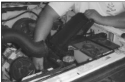
8. Disconnect the air inlet from the airbox base and remove the airbox base.
