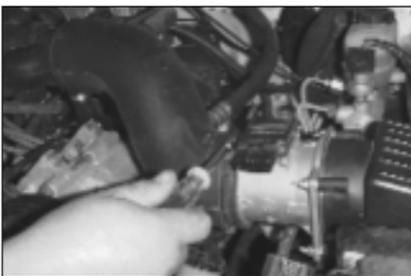
5. Loosen the hose clamp at the mass air sensor.
