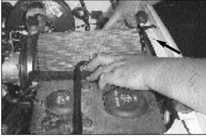
19. Reinstall the Filtercharger element and secure the bracket with the hardware provided.
