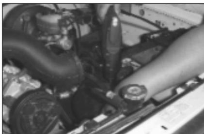
9. Drill a hole through the air inlet tube and inner fender.
