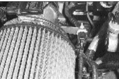
21. Insert the air temperature sensor into the bracket as shown.
