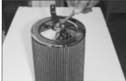
15. Using the hardware provided, install and secure the bracket onto the end of the Filtercharger element.
