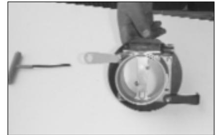
12. Secure the mass air sensor adaptor to the mass air sensor using the rubber gasket and hardware provided, with brackets positioned as shown.
