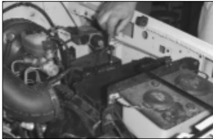
7. Loosen the two bolts that secure the airbox base.
