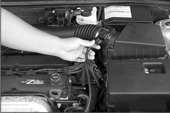
2. Disconnect the mass air electrical connection
