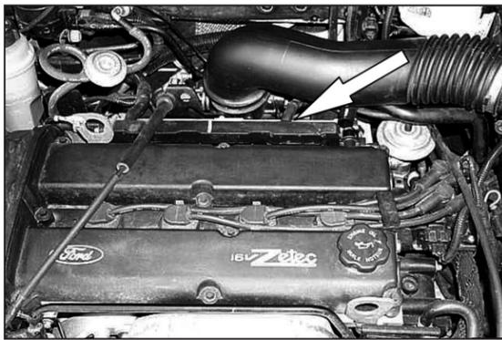
4. Disconnect the vent hose from the valve cover.
