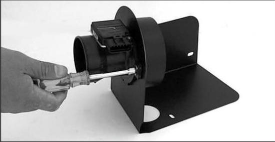
11. Assemble the mass air sensor, heat shield & filter adapter with hardware provided
