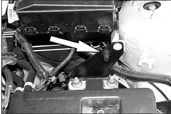
6. Remove rubber bumper from the air box mounting location.
