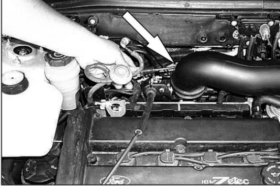
3. Loosen the hose clamp at the throttle body.
