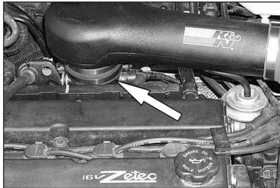
18. Install the new air intake tube onto the throttle body, then tighten all the hose clamps.
