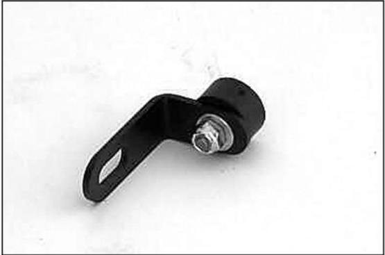
8. Install the rubber-mounted stud onto the "L" bracket as shown above.
