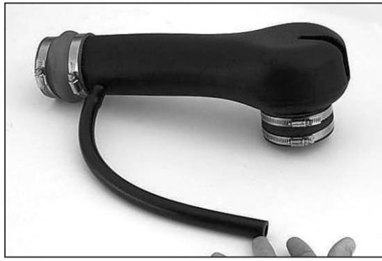
16. Install the silicone vent hose onto the new intake tube as shown.
