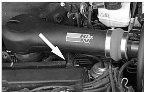
19. Install the silicone vent hose onto the valve cover.
