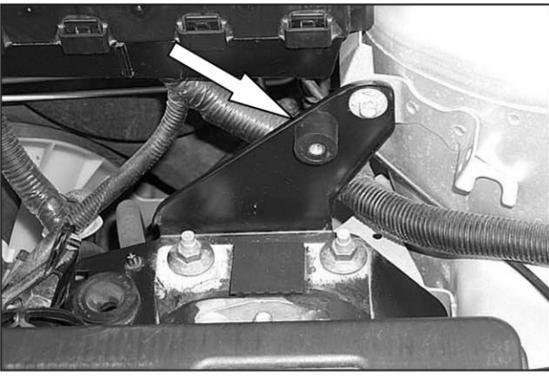
10. Install the rubber-mounted stud onto the existing air box-mounting tray.
