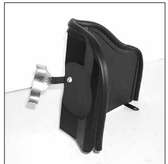
10. Install saddle bracket assembly onto heat shield as shown. Do not tighten completely.
