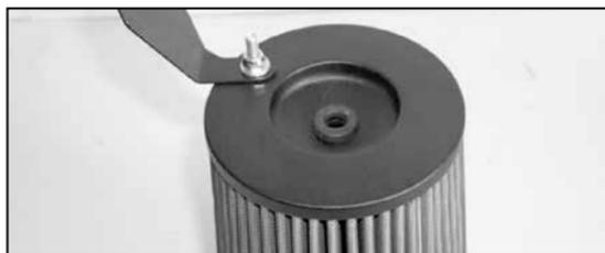
23. Install grommet into new Air Filter top as shown.
