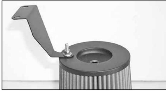
20. Install filter bracket onto filter as shown, but do not tighten completely.
