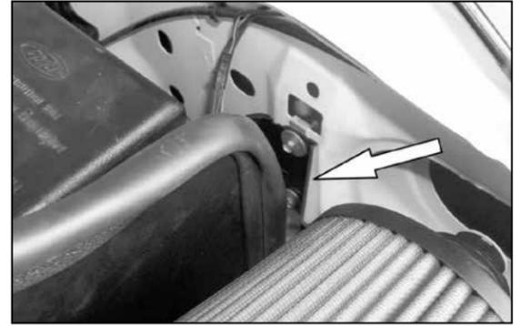
26. Now install the new filter bracket behind the fuse box mounting bracket as shown.
