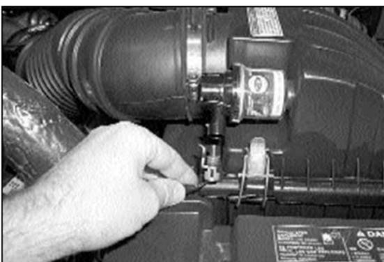
2. On 2002 models disconnect the restrictor gauge electrical connection as shown.
