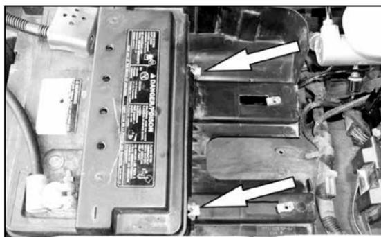
7. Remove the two upper airbox mounting clips.
