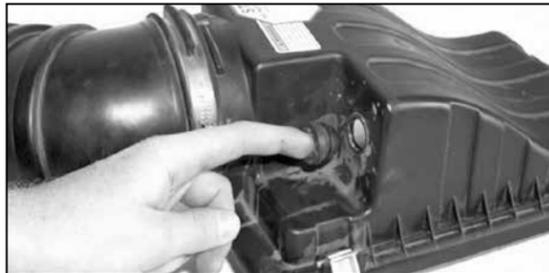
22. Remove restriction gauge grommet from stock airbox top.
