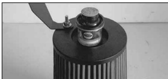
24. Install filter restriction gauge onto Air Filter top as shown.
