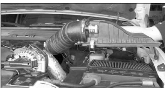
3. Loosen the hose clamp at the intake manifold. Release the clips from airbox top then remove complete upper intake.
