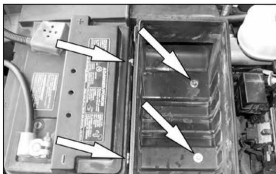
5. Loosen and remove the 4 bolts that retain the stock airbox.
