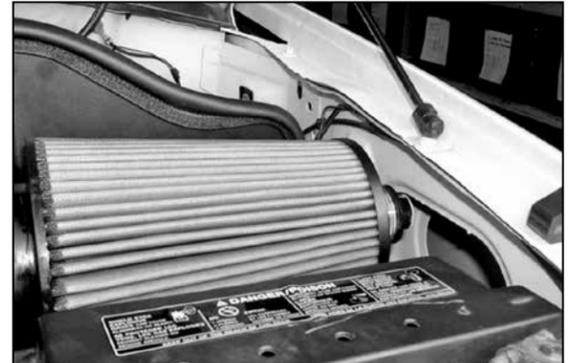
27. Adjust all brackets to obtain maximum clearance for intake tube and Air Filter element then tighten completely.
