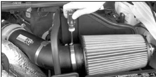
25. Install Air Filter onto intake tube as shown but do not tighten completely.
