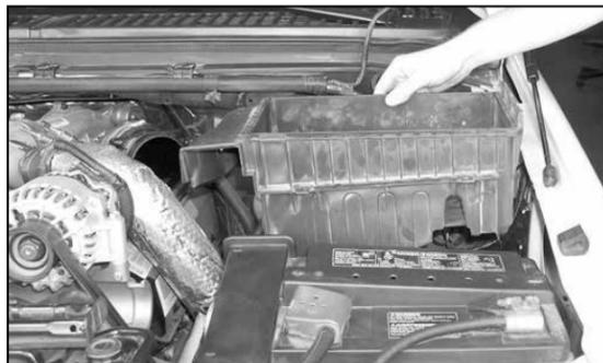
6. Then remove the stock airbox base from vehicle.
