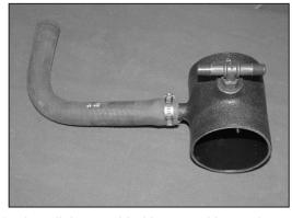
15. Install the provided hose and hose clamp onto the  $K\&N^{\otimes}$  intake tube as shown.
