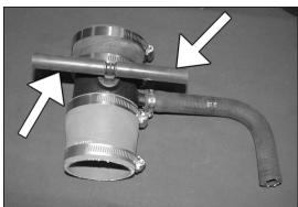
18. Install the two provided hoses onto the "T" vent on the K&N® intake tube as shown.
