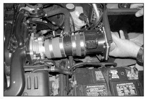
20. Install the  $K\&N^{\scriptsize @}$  intake assembly onto the throttle body as shown.
