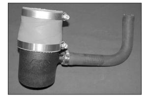
16. Assemble the large silicone step hose and hose clamps onto the  $K\&N^{\tiny \circledcirc}$  intake tube as shown.
