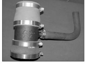
17. Assemble the small silicone step hose and hose clamps onto the  $K\&N^{\scriptsize \circledcirc}$  intake tube as shown.
