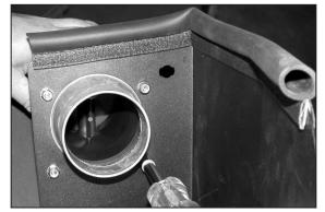
13. Slide the mass air assembly into the bolt pattern on the heat shield, then, secure it with the provided hardware as shown.
