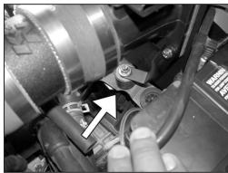
21. Line up the twist bracket with the rubber mounted stud, and secure it with the provided hardware as shown.
