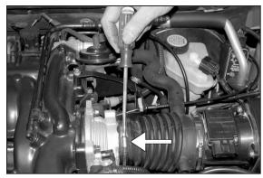
5. Loosen the hose clamp at the throttle body as shown.
