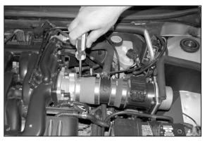
22. Adjust the tube and silicone hoses for best fit, then, tighten the hose clamps as shown.
