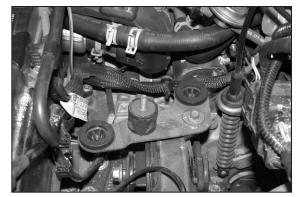
8. Install the provided rubber mounted stud to the threaded hole from step 7.
