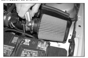
29. Install the K&N® air filter and secure it with the provided hose clamp as shown.
