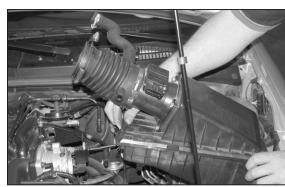
6. Remove the rubber intake hose from the throttle body, then, pull firmly upwards to release the air cleaner assembly from the stock grommets as shown.
