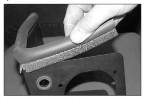
12. Apply the edge trim onto the heat shield as shown. Trim excess if necessary.
