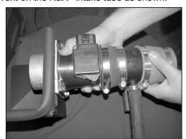
19. Install the K&N® intake tube assembly onto the heat shield assembly as shown.
