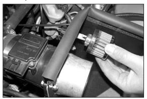
27. Install the provided  $K\&N^{\scriptsize @}$  vent filter onto the air temperature sensor as shown.
