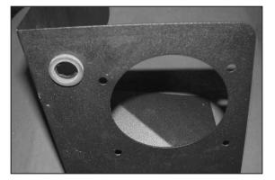
11. Apply the provided adhesive back gasket to the key-hole on the heat shield as shown.
