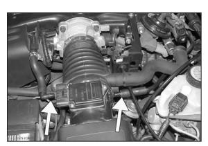
4. Disconnect the crank case vent hoses and the IAC vent hose as shown.
