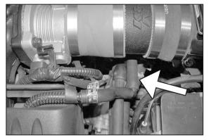
25. Reconnect the crank case vent hose as shown.
