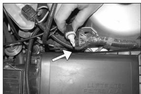
3. Turn the air temperature sensor  $\frac{1}{4}$  turn, then pull it out of the air cleaner assembly to remove as shown.
