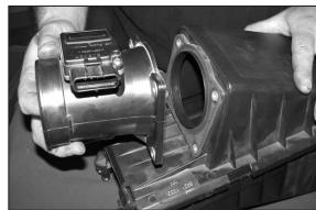
9. Loosen and remove the four bolts that secure the mass air sensor to the air cleaner, then, remove the mass air sensor as shown.
