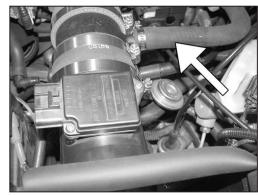
24. Reconnect the crank case vent hose as shown.
