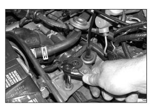
7. Loosen and remove the stock hex bolt from the air cleaner support bracket as shown.
