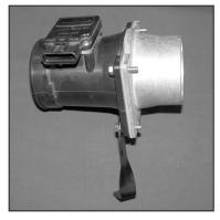
10. Assemble the mass air adapter, gasket, mass air sensor, and the twist bracket using the provided hardware as shown.
