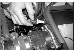
26. Install the air temperature sensor into the keyhole in the heat shield as shown. Turn it ½ turn to lock into place.
