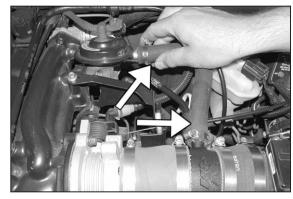
23. Reconnect the IAC vent and tighten with the provided hose clamp as shown.
