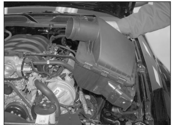
6. Remove the airbox assembly as shown.
