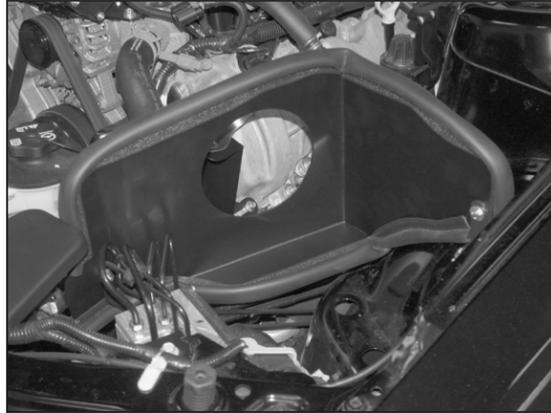
13. Install the heat shield and secure with the provided hardware as shown.
