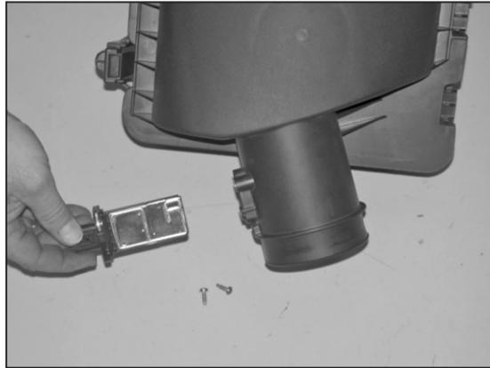
14. Remove the mass air sensor from the factory airbox with the T20 "TORX" wrench provided.
