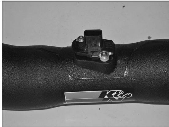
15. Install the mass air sensor into the K&N® intake tube with the mounting screws and two spacers provided.
