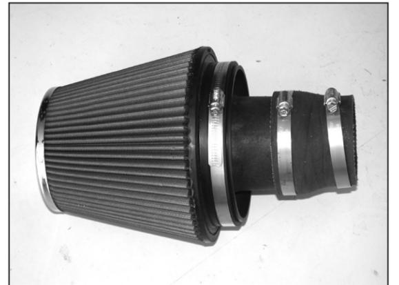
21. Install the silicone hose (08724) onto the air filter assembly and secure with the provided hose clamp as shown.
