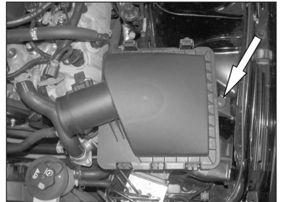
5. Remove the airbox mounting bolt shown.
