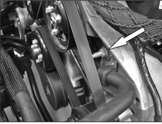
7. Remove the power steering pump bracket-retaining nut shown.
