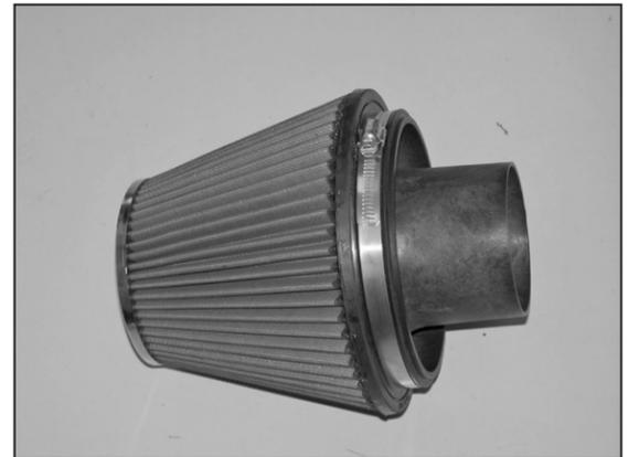
20. Install the air filter onto the filter adapter and secure with the provided hose clamp as shown. **NOTE: Drycharger® air filter wrap; part # RF-1048DK is available to purchase separately. To learn more about Drycharger® filter wraps or look up color availability please visit <http://www.knfilters.com>.**
