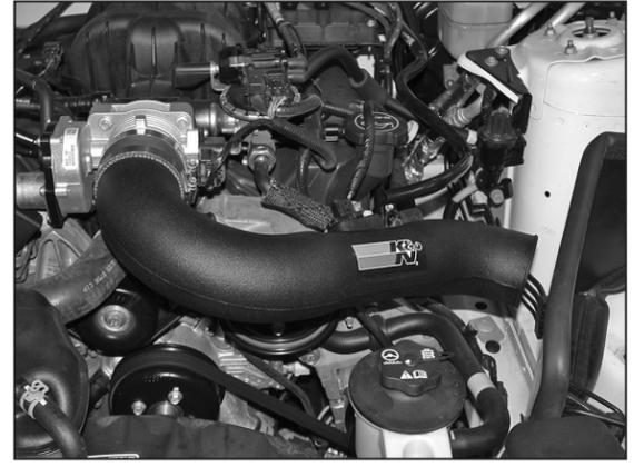
17. Install the K&N® intake tube into the silicone hose at the throttle body and onto the tube-mounting bracket installed in step #8, secure with provided hardware.
