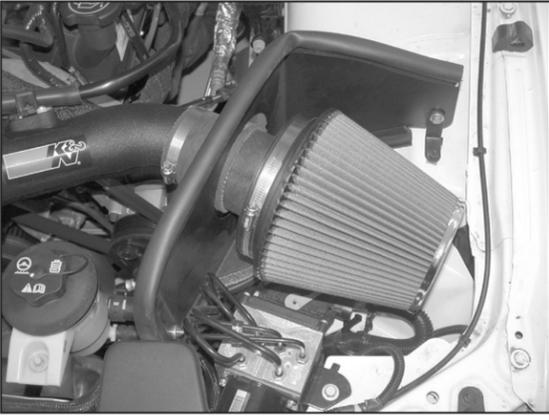
22. Install the air filter assembly onto the K&N® intake tube as shown and secure with the provided hose clamp.
