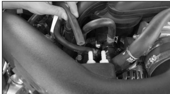
29. Install the supplied shorter crank case vent line onto the fitting on the valve cover and then onto the npt fitting installed in the K&N® intake tube.
