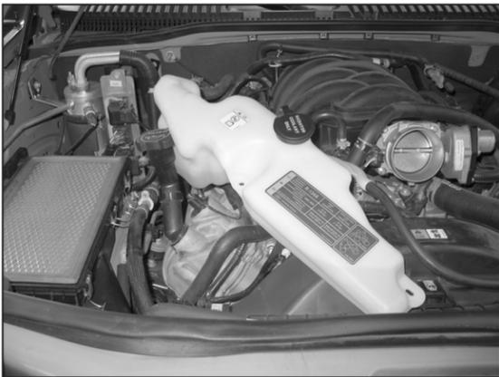
9. Lift and position the coolant recovery tank on the engine to gain access to the lower air box.
