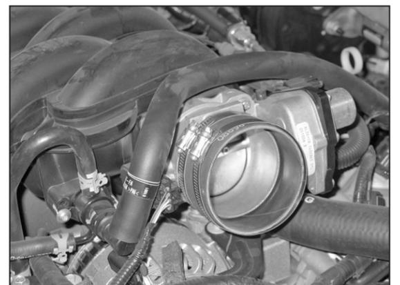
22. Install the silicone hose (08630) onto the throttle body and secure with the provided hose clamp.
