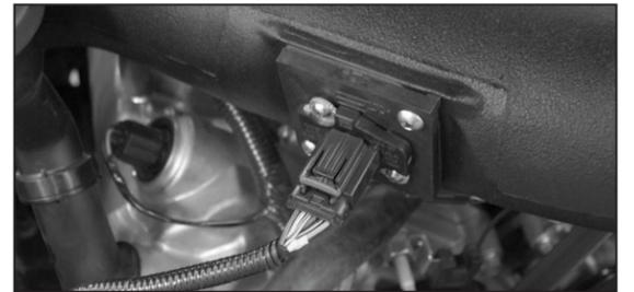
34. Reconnect the mass air sensor electrical connection.
