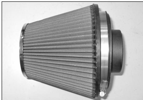
31. Install the filter adapter into the K&N® air filter as shown and secure with the provided hose clamp.
