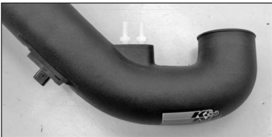
27. Install the two npt vent fittings into the K&N® intake tube as shown.
