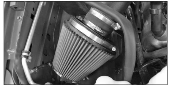
33. Install the air filter assembly onto the K&N intake tube and secure with the provided hose clamp.
