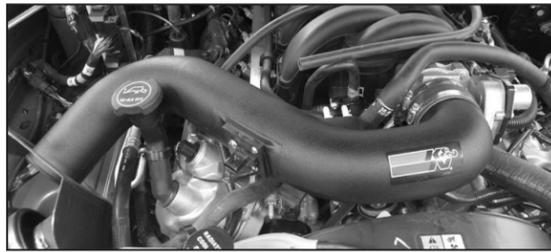
28. Install the K&N® intake tube into the silicone hose at the throttle body and align with the mounting bracket installed in step #16. Secure the intake tube with the hose clamp and supplied hardware.
