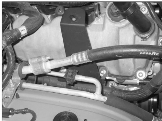
16. Install the tube mounting bracket onto the valve cover and secure with the factory valve cover mounting bolt and the supplied hardware as shown.
