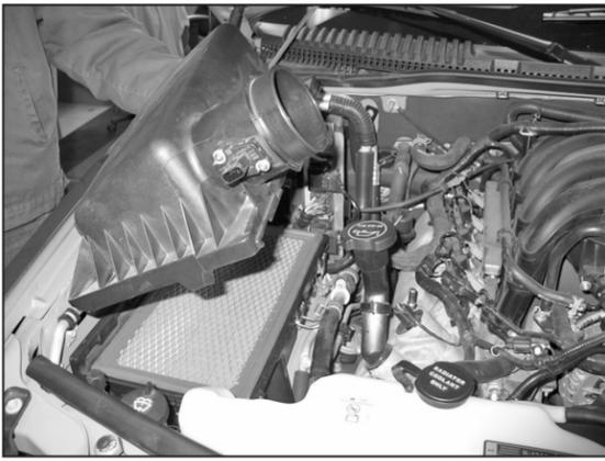
7. Unlatch the three air box lid latches and then remove the lid from the vehicle
