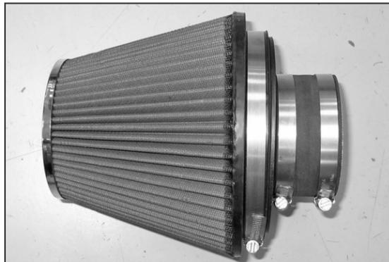
32. Install the silicone hose (08630) onto the air filter adapter and secure with the provided hose clamp.
