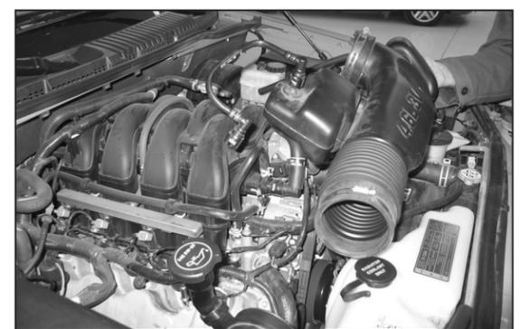
6. Remove the stock intake tube from the vehicle as shown.
