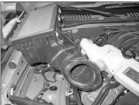
10. Lift up the lower air box housing to dislodge it from the mounting grommets and then remove the lower air box housing from the vehicle.
