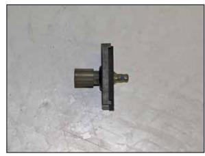
19. Remove the O-Ring from the sensor and then install the sensor into the grommet installed into the adapter as shown.
