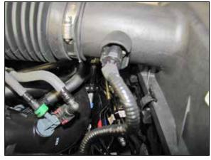
2. Depress the locking tab and then disconnect the inlet air temperature sensor electrical connection.
