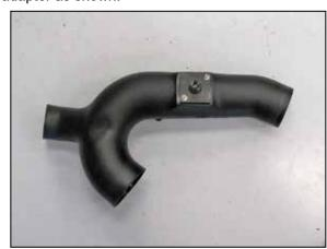
20. Install the inlet air temperature sensor assembly into the  $K\&N^{@}$  intake tube and secure with the provided hardware.
