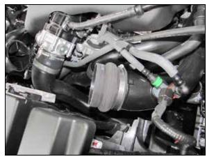
13. Install the provided hump coupler (08418) onto the driver's side turbo inlet tube.
