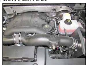
21. Install the K&N® intake tube into the coupling hoses and then secure with the provided hose clamps.
