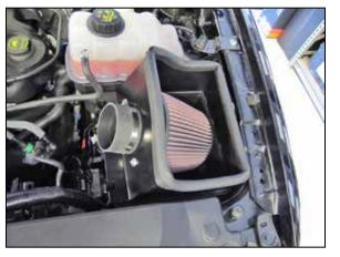
12. Install the heat shield assembly onto the lower air filter housing and secure with the factory retaining clip.
