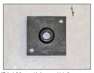
17. Install the provided grommet into the temperature sensor adapter as shown.
