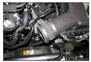
10. Install the provided coupler hose (08633) onto the air filter housing and secure with the provided hose clamp.
