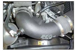
12. Install the K&N® intake tube assembly into the coupler hoses, adjust for best fit and then secure with the provided hose clamps. Connect the factory vent lines to the fittings installed into the intake tube.
