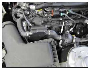
5. Remove the clamp that secures the sound tube to the sound drum and then remove the sound
