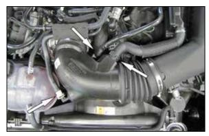
3. Disconnect the EVAP, crank case and sound tube vent lines from the intake tube.
